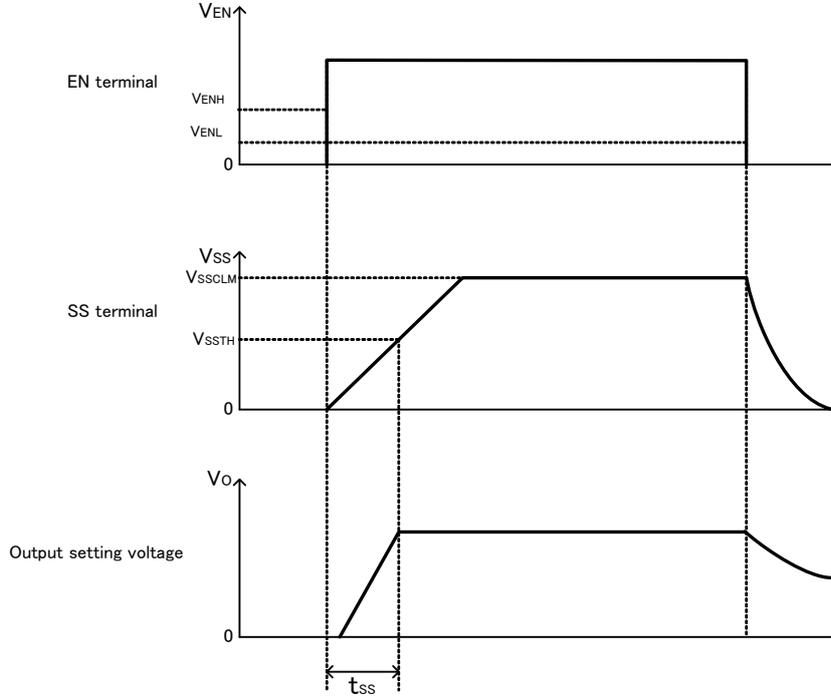
Fig.12 ON/OFF transition wave form in EN controlling
