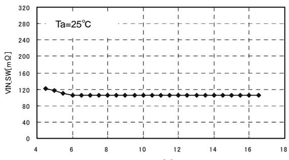
Fig.9 Hi side FET ON\_R - VIN characteristic
