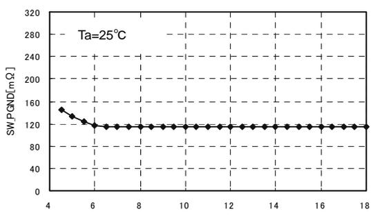
Fig.10 Low side FET ON\_R – VIN characteristic
