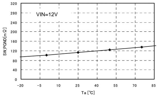
Fig.8 Low side FET ON\_R - temperature characteristic
