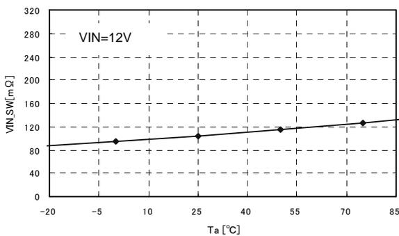
Fig.7 Hi side FET ON\_R - temperature characteristic
