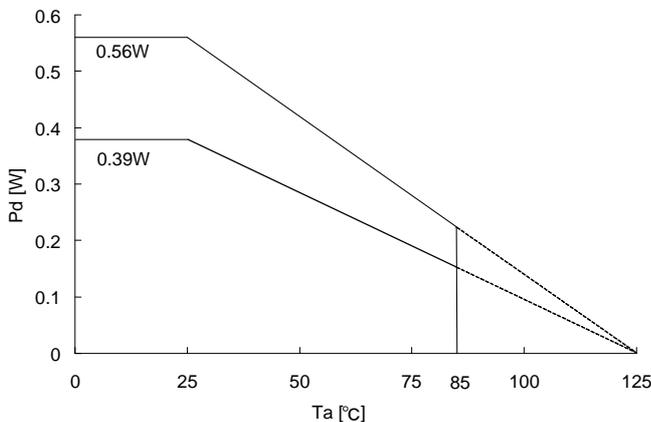
\* Please design the margin so that P<sub>MAX</sub> becomes is than Pd (P<sub>MAX</sub><Pd) within the usage temperature range
