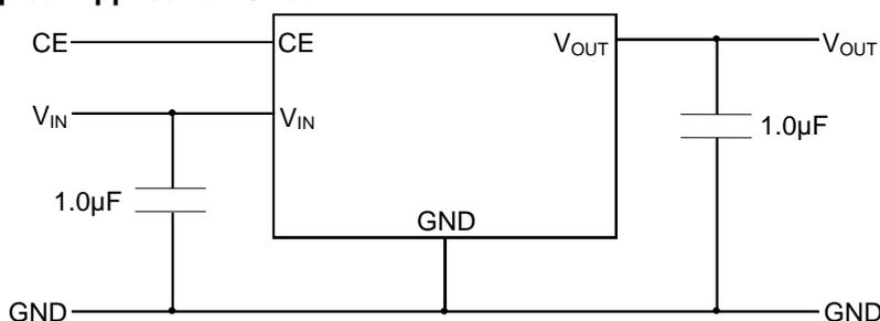
Figure 1. Application Circuit
