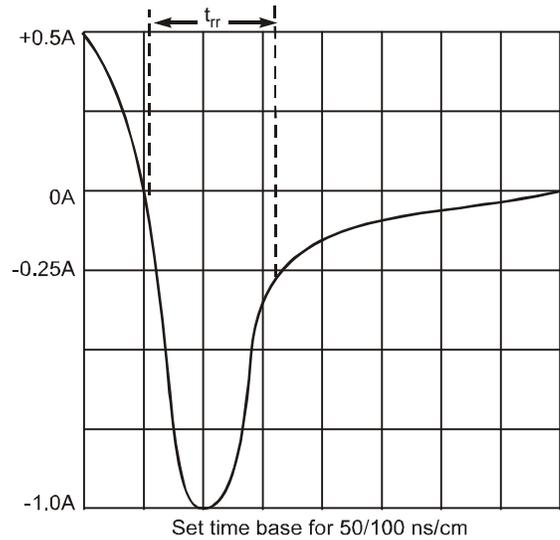
Fig. 5 Reverse Recovery Time Characteristic and Test Circuit
