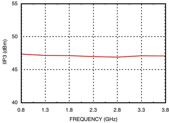
**Input IP3 vs. Frequency @ VDD= 5V,
