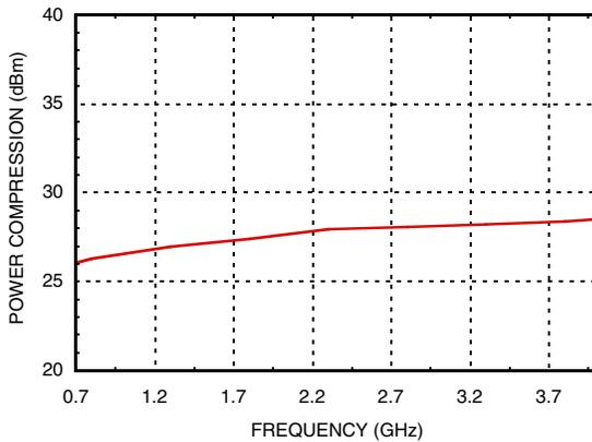
**P0.1dB Vs. Frequency @ VDD= 5V,
