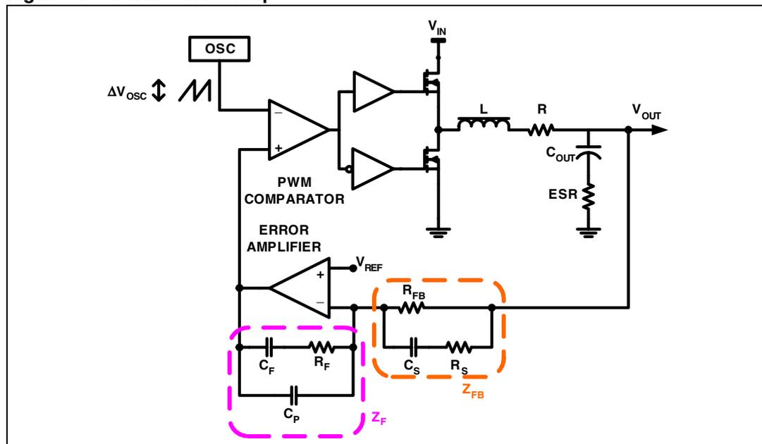
The compensation network closes the loop joining  $V_{OUT}$  and EA output with transfer function ideally equal to  $-Z_F/Z_{FB}$ .
