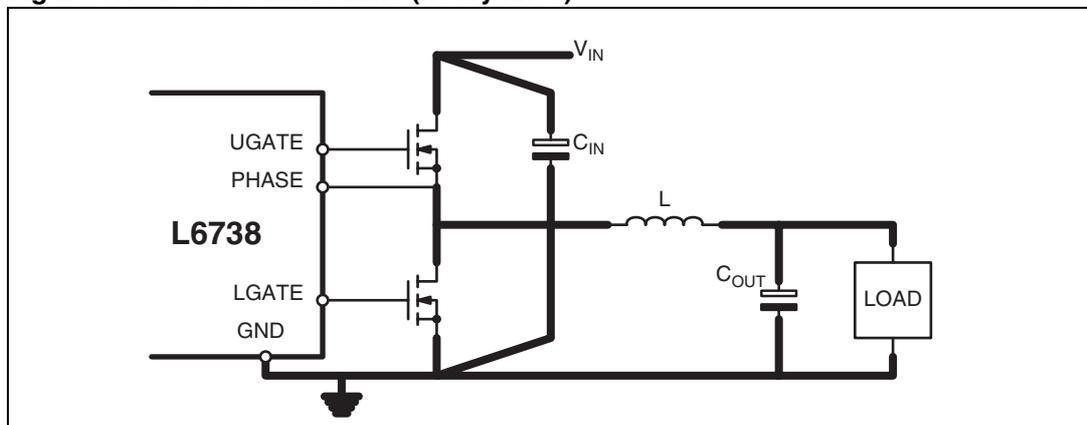
Gate traces and phase trace must be sized according to the driver RMS current delivered to the Power MOSFET. The device robustness allows the managing of applications with the power section far from the controller without losing performance. However, when possible, it is recommended to minimize the distance between the controller and power section.
