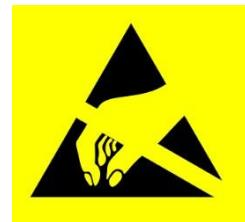
**Observe precautions for handling electrostatic sensitive devices.**
