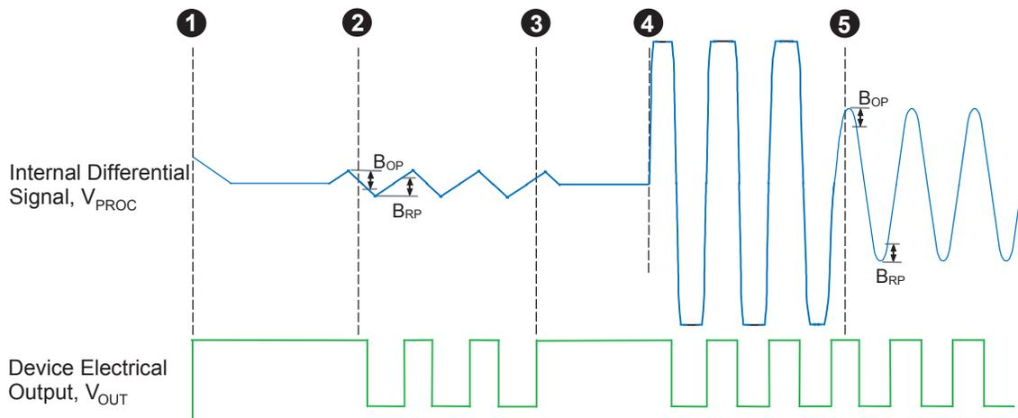
Figure 7: Operation of Running Mode Gain Adjust
