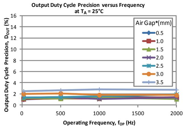
\*Air gap defined as the distance between the front face of the A1468 package and the Allegro Reference Target 60-0 ring magnet
