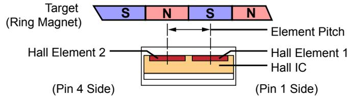
**Figure 1: Relative Motion of the Target**
