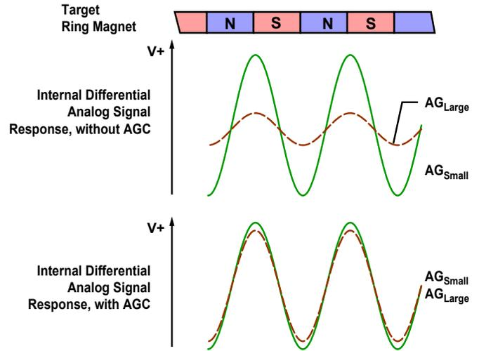
**Figure 4: Automatic Gain Control (AGC)**
