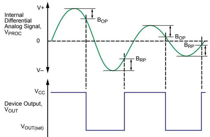
**Figure 5: Differential Signal Peaks**
