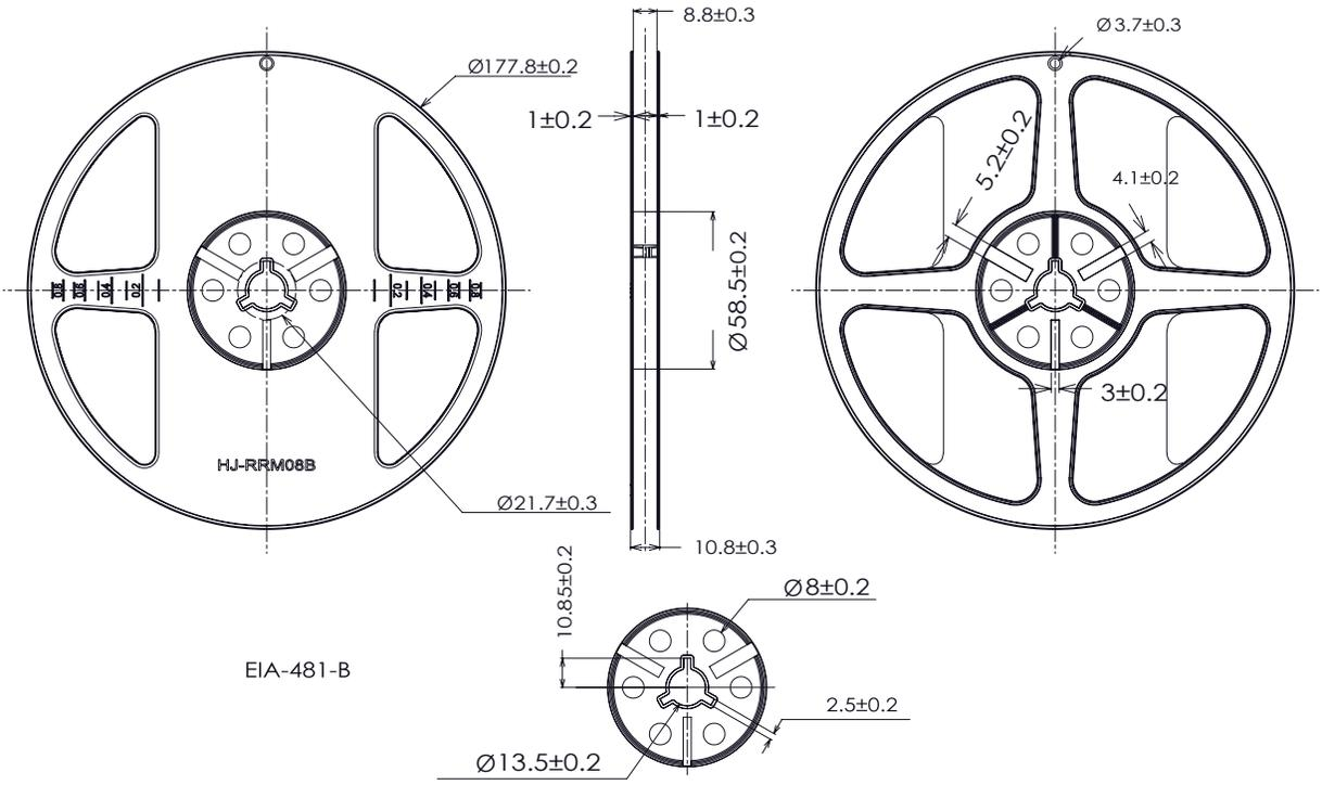
Figure 11. Reel dimensions for LUXEON 2835 Commercial.
