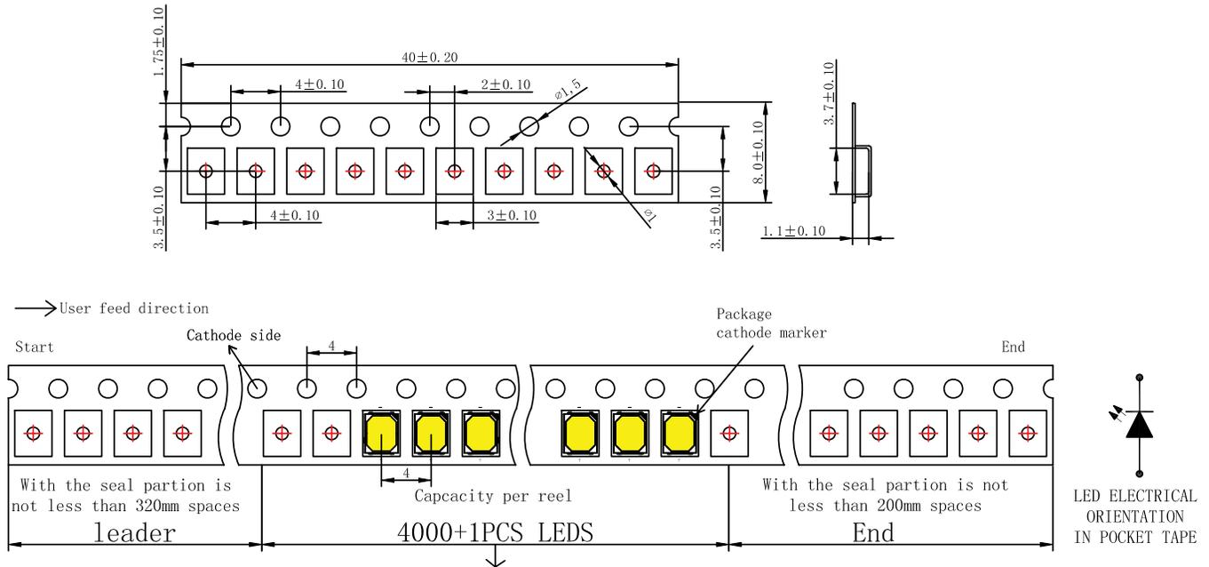
Figure 10. Pocket tape dimensions for LUXEON 2835 Commercial.
