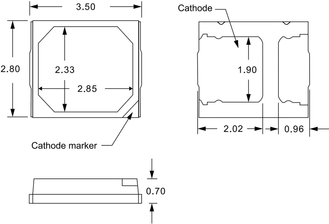
Figure 7. Mechanical dimensions for LUXEON 2835 Commercial.
