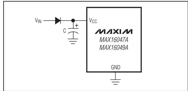
Figure 15. Power Circuit for Shutdown During Fault Conditions
