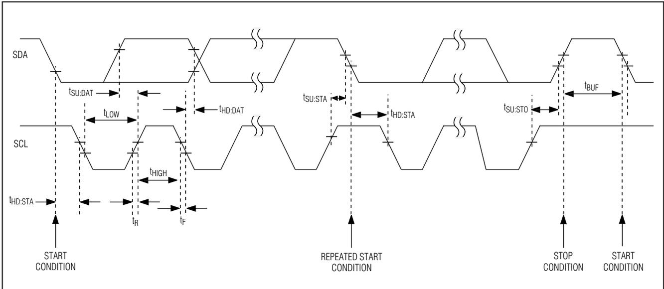
Figure 1. I<sup>2</sup>C/SMBus Timing Diagram
