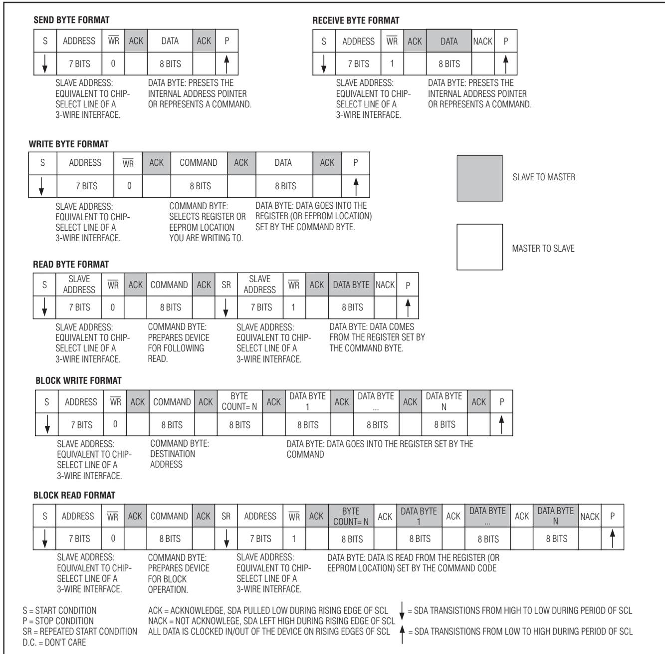
Figure 12. I<sup>2</sup>C/SMBus Protocols
