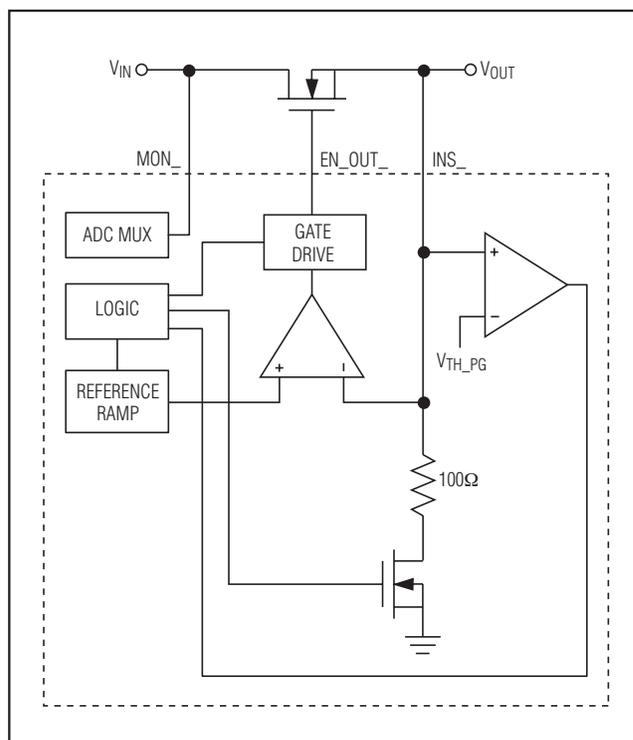
Figure 5. Closed-Loop Tracking
