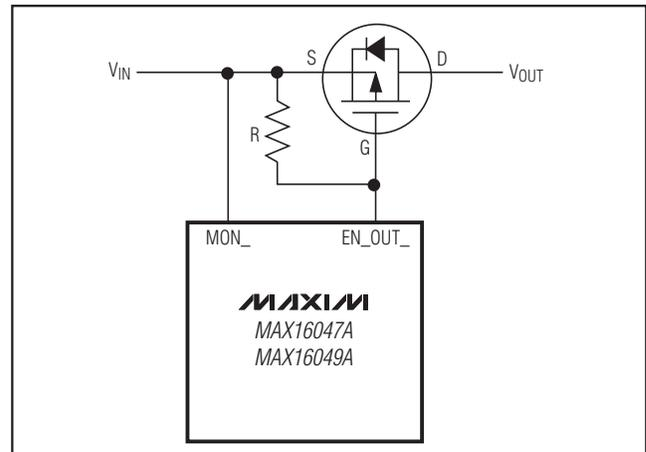
Figure 17. Connection for a p-Channel Series-Pass MOSFET
