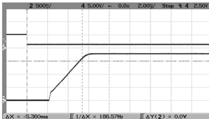
Step Load Transient Response (VIN=5V, V<sub>OUT</sub>=1.8V, I<sub>OUT</sub>=6A to 3A)
