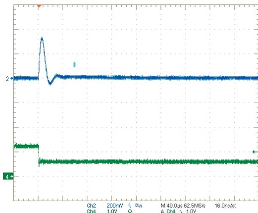
Step Load Transient Response (VIN=5V, V<sub>OUT</sub>=1.8V, I<sub>OUT</sub>=3A to 6A)
