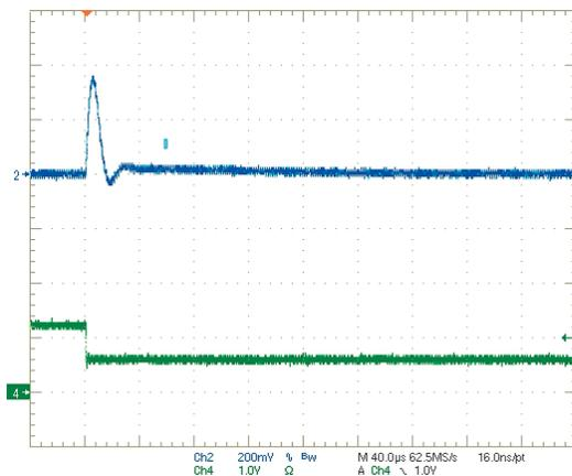
Step Load Transient Response (V<sub>in</sub>=5V, V<sub>out</sub>=2.5V, I<sub>out</sub>=3A to 6A)
