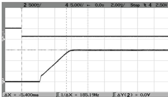
Step Load Transient Response (VIN=5V, V<sub>OUT</sub>=1.5V, I<sub>OUT</sub>=6A to 3A)
