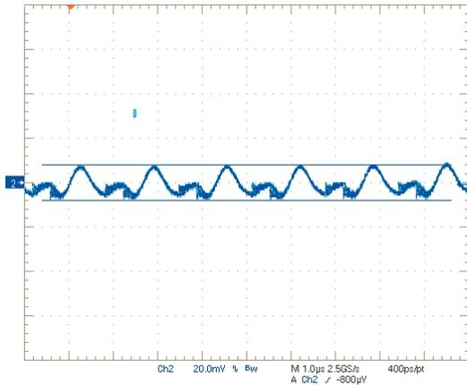
On/Off Enable Startup (V<sub>in</sub>=5V, V<sub>out</sub>=1.0V, I<sub>out</sub>=6A, Cload=0)
