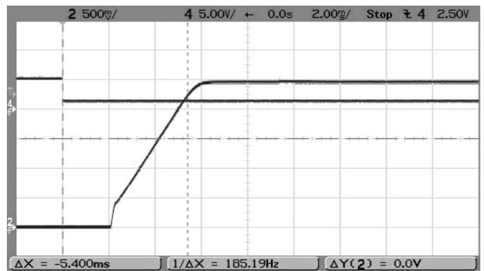
Step Load Transient Response (V<sub>in</sub>=5V, V<sub>out</sub>=2.5V, I<sub>out</sub>=6A to 3A)
