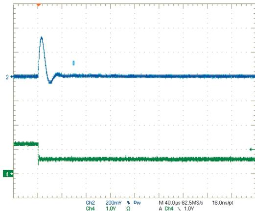
Step Load Transient Response (V<sub>in</sub>=5V, V<sub>out</sub>=1.2V, I<sub>out</sub>=3A to 6A)
