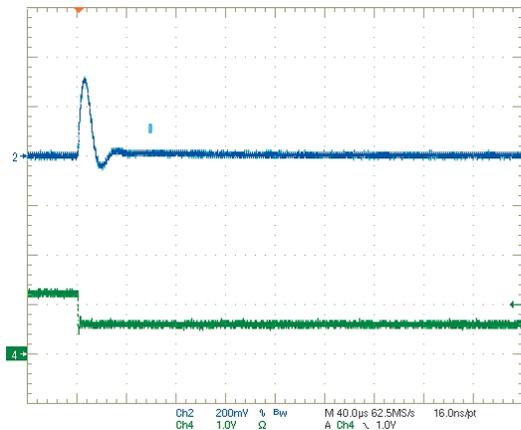
Step Load Transient Response (VIN=5V, V<sub>OUT</sub>=1.5V, I<sub>OUT</sub>=3A to 6A)
