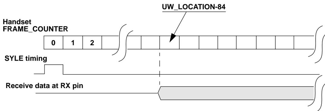
**Figure 7. Frame Counter and UW\_LOCATION on Handset**
