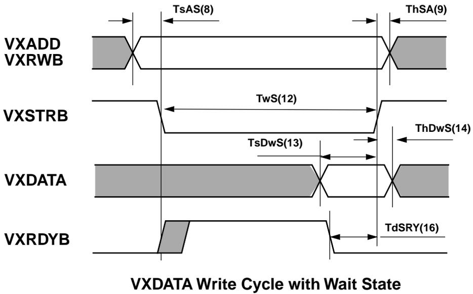
Figure 9. Read/Write Cycle Timing with Wait State
