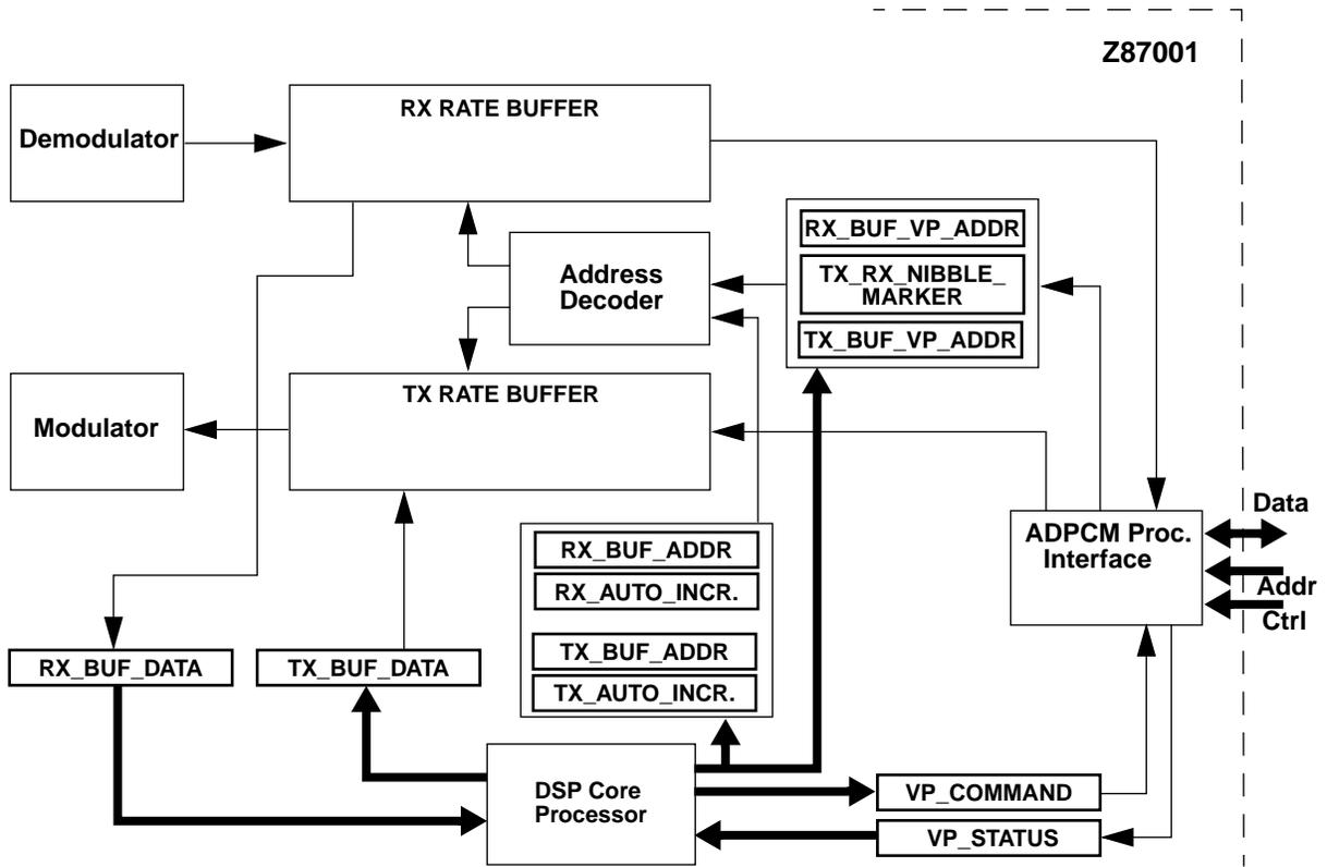
Figure 9. Rate Buffers Access and ADPCM Processor Interface
