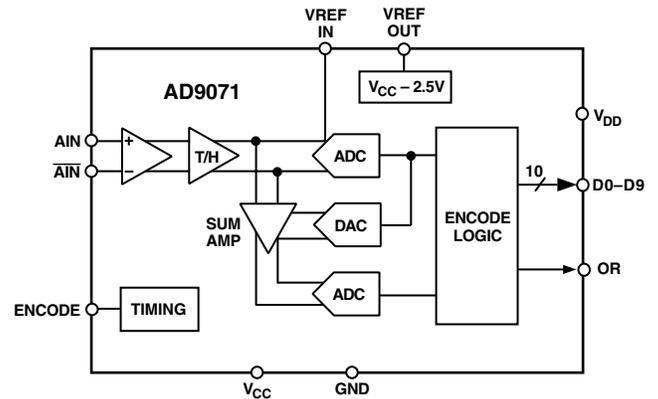
interfacing with 3.3 V or 5 V logic. An out-of-range output (OR) is available that indicates a conversion result is outside the operating range. The output data are held at saturation levels during an out-of-range condition.
