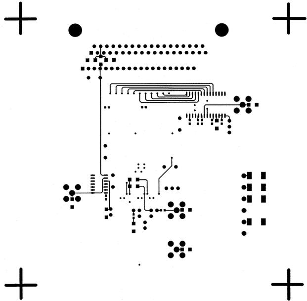
Figure 15. Printed Circuit Board Bottom Side Copper
