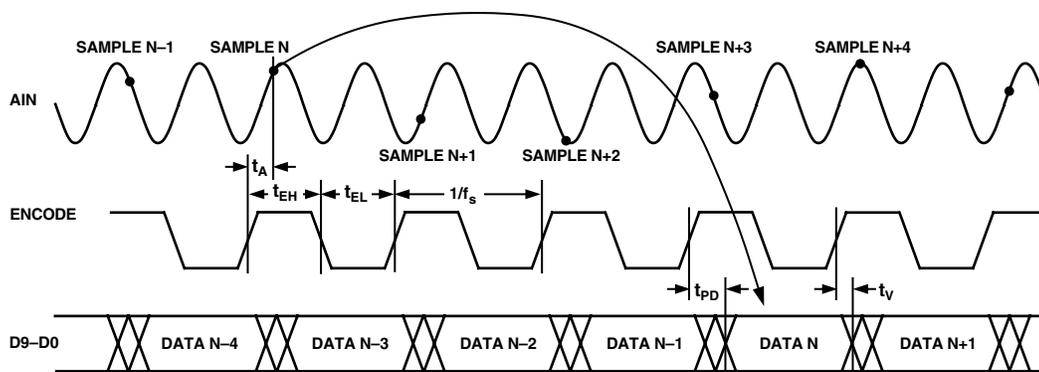
Figure 1. Timing Diagram
