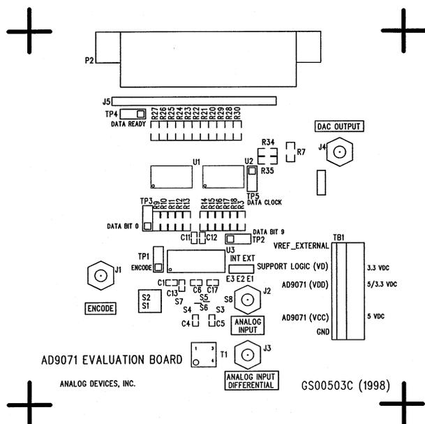
Figure 10. Printed Circuit Board Top Side Silkscreen
