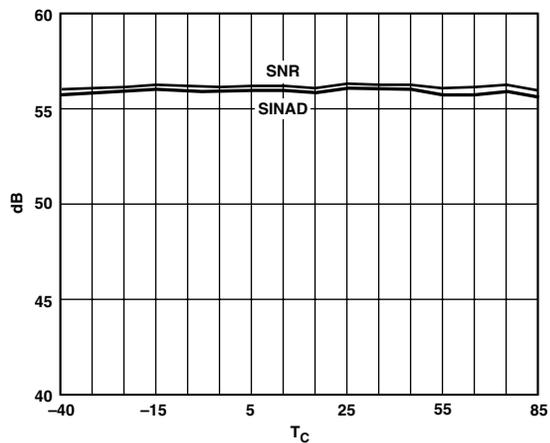
TPC 7. Differential SNR vs.  $T_C$ :  $f_{IN} = 10.3$  MHz
