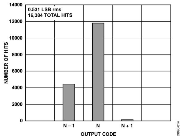
Figure 15. AD9634-170 Grounded Input Histogram,  $f_s = 170$  MSPS
