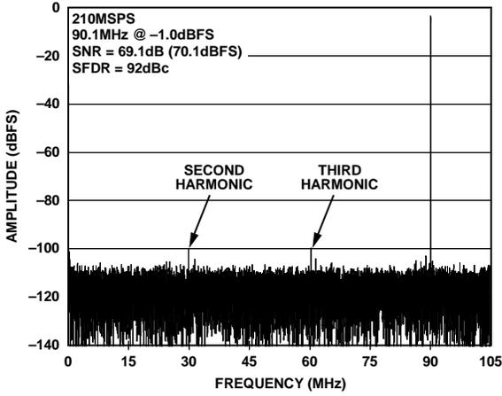
Figure 16. AD9634-210 Single-Tone FFT with  $f_{IN} = 90.1$  MHz
