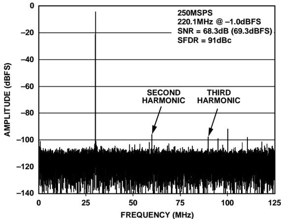
Figure 30. AD9634-250 Single-Tone FFT with  $f_{IN} = 220.1$  MHz
