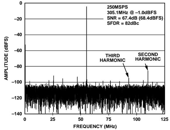
Figure 31. AD9634-250 Single-Tone FFT with  $f_{IN} = 305.1$  MHz
