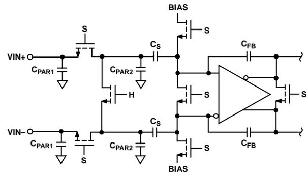
Figure 46. Switched-Capacitor Input
