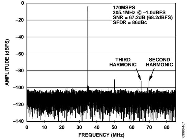
Figure 7. AD9634-170 Single-Tone FFT with  $f_{IN} = 305.1$  MHz
