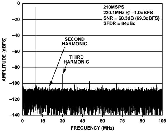
Figure 18. AD9634-210 Single-Tone FFT with  $f_{IN} = 220.1$  MHz
