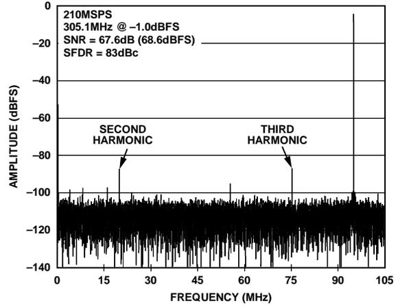
Figure 19. AD9634-210 Single-Tone FFT with  $f_{IN} = 305.1$  MHz
