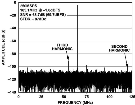
Figure 29. AD9634-250 Single-Tone FFT with  $f_{IN} = 185.1$  MHz
