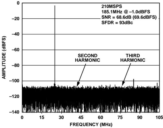
Figure 17. AD9634-210 Single-Tone FFT with  $f_{IN} = 185.1$  MHz
