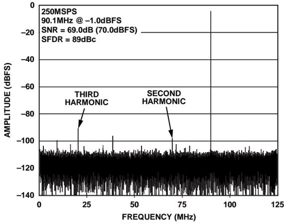
Figure 28. AD9634-250 Single-Tone FFT with  $f_{IN} = 90.1$  MHz
