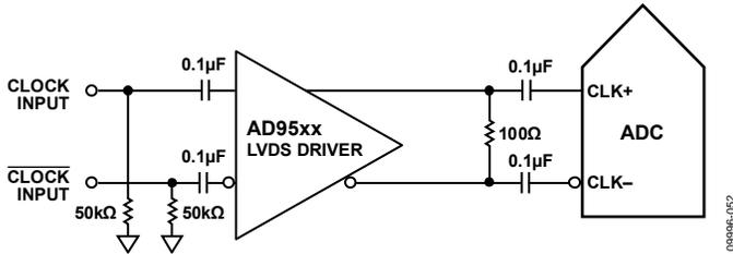
Figure 55. Differential LVDS Sample Clock (Up to 625 MHz)
