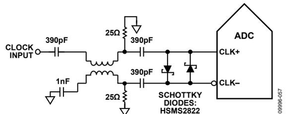
Figure 53. Balun-Coupled Differential Clock (Up to 625 MHz)
