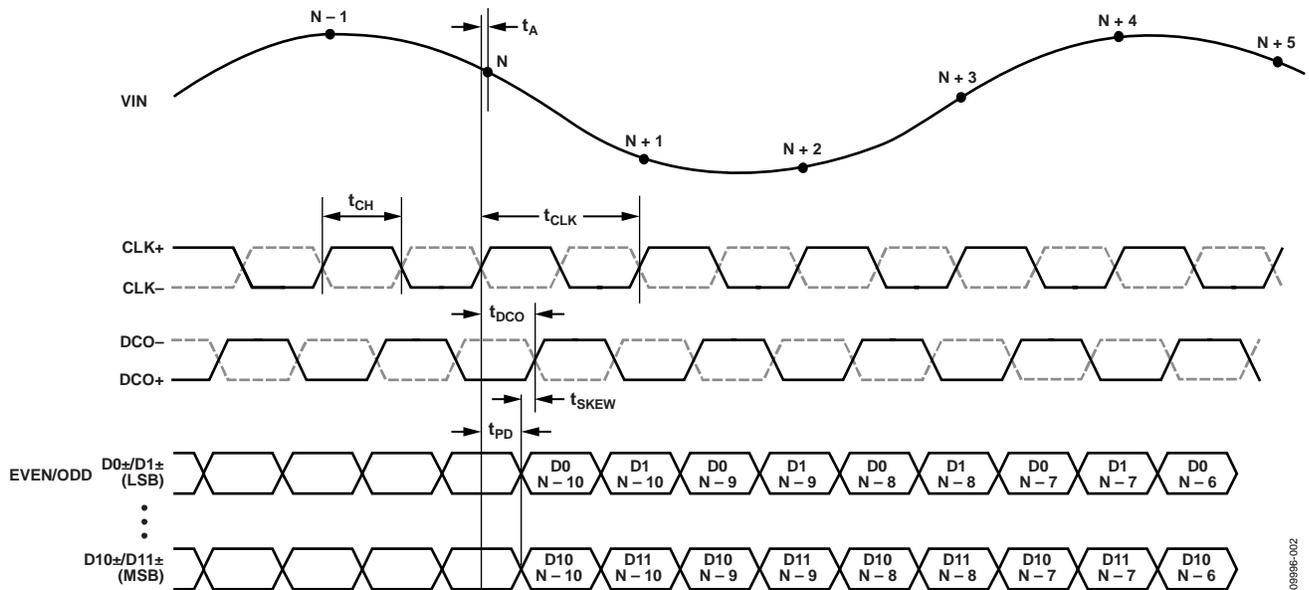
Figure 2. Even/Odd LVDS Mode Data Output Timing
