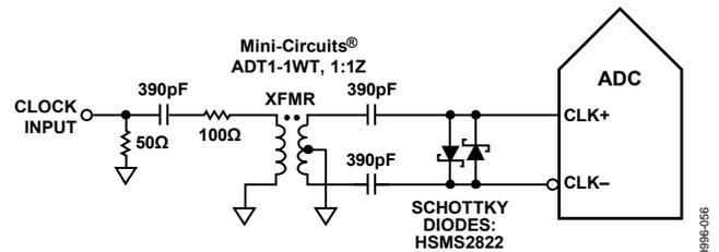
Figure 52. Transformer Coupled Differential Clock (Up to 200 MHz)
