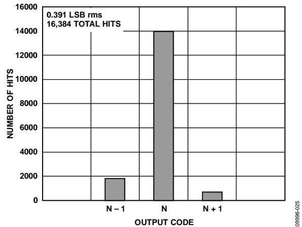
Figure 27. AD9634-210 Grounded Input Histogram,  $f_s = 210$  MSPS
