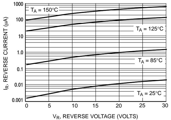
Figure 3. Leakage Current
