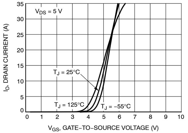
Figure 2. Transfer Characteristics
