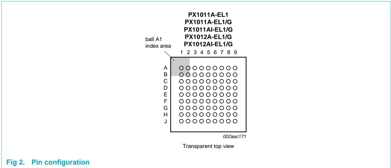
Fig 2. Pin configuration
