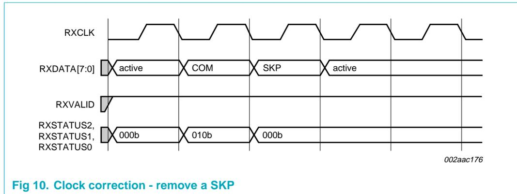
Fig 10. Clock correction - remove a SKP
