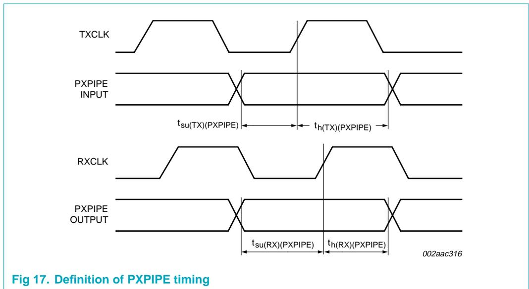
**Fig 17. Definition of PXPIPE timing**
