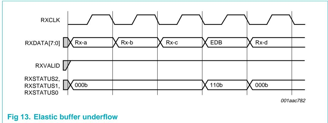
Fig 13. Elastic buffer underflow
