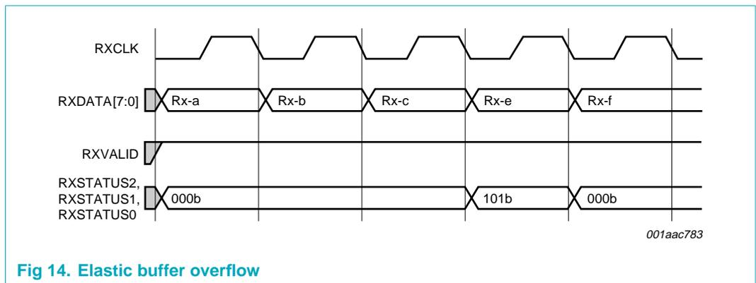
Fig 14. Elastic buffer overflow
