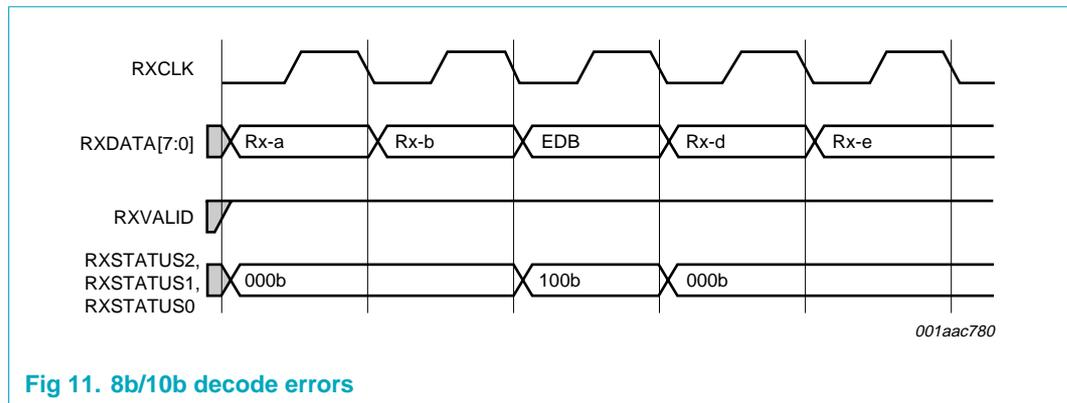
**Fig 11. 8b/10b decode errors**
