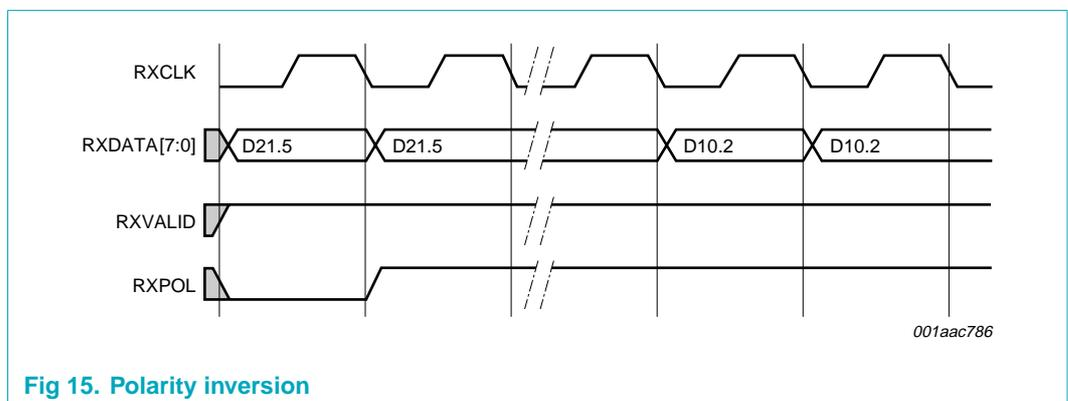
Fig 15. Polarity inversion
