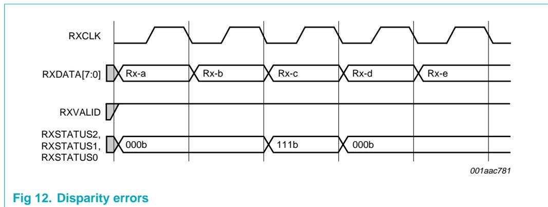
**Fig 12. Disparity errors**
