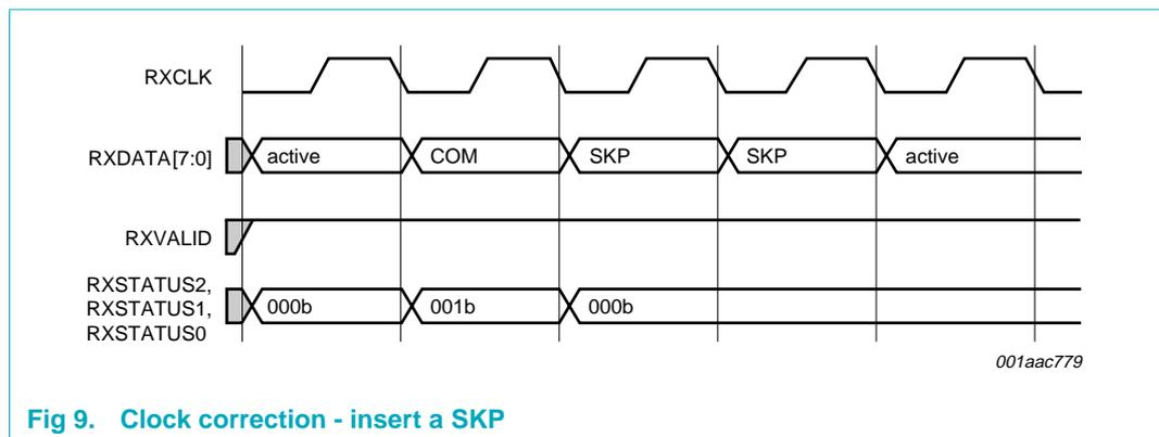
Fig 9. Clock correction - insert a SKP
