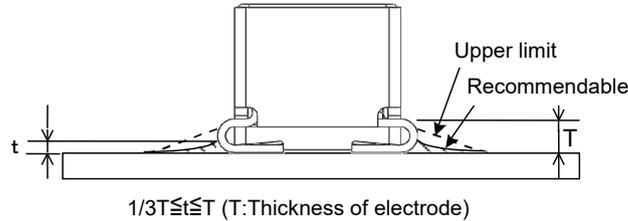
Accordingly increasing the solder volume, the mechanical stress to Chip is also increased. Exceeding solder volume may cause the failure of mechanical or electrical performance. In case if the solder volume is much, we recommend to make the size of the solder paste with less than the land pattern.
