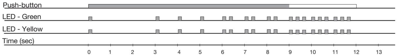
Releasing the push-button after 12 sec. returns the sensor to factory settings.
