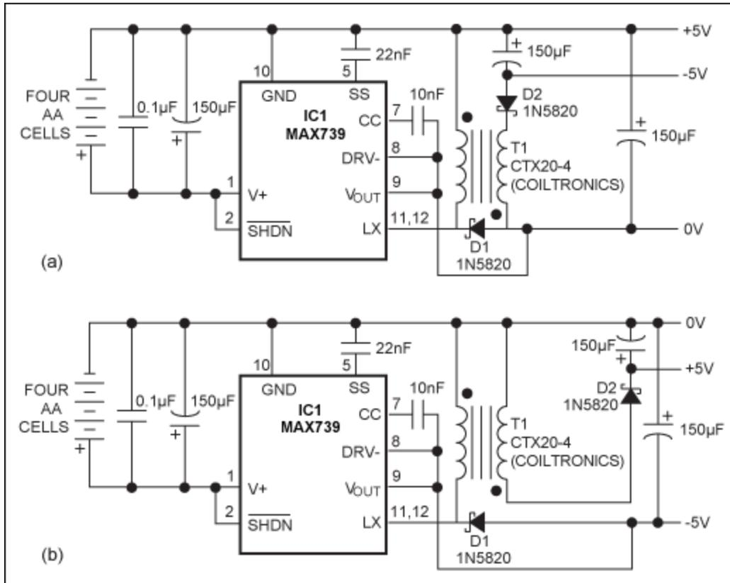
Figure 1. A 1:1 transformer enables this inverting switching regulator to generate -5V (a). Different connections for the right-hand coil are recommended if -5V supplies the heavier load current (b).
