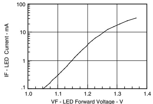
Fig. 4 - LED Forward Current vs. Forward Voltage
