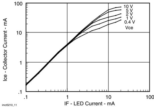
Fig. 11 - Collector Current vs. LED Current
