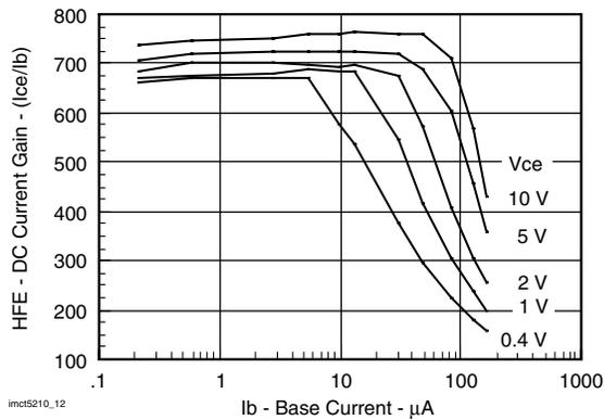
Fig. 12 - Transistor Current Gain vs. Base Current
