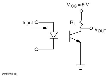
Fig. 1 - Switching Schematic
