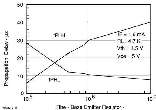
Fig. 16 - Propagation Delay vs. Base Emitter Resistor
