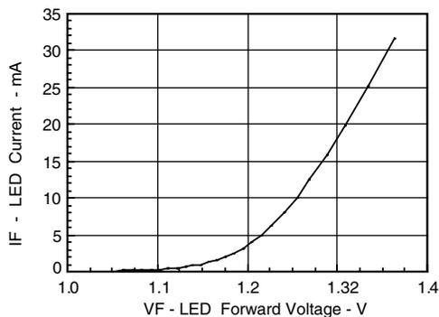
Fig. 3 - Forward Current vs. Forward Voltage
