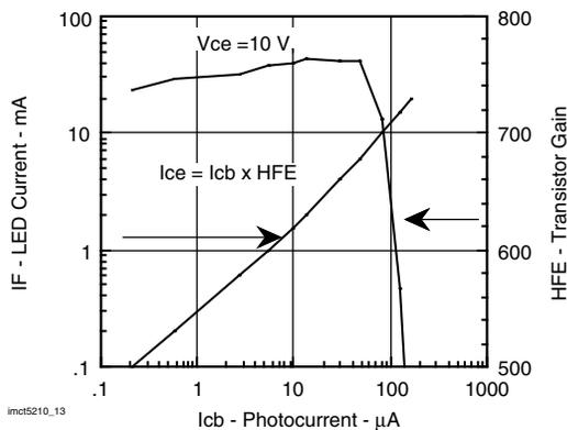
Fig. 13 - Transfer Curve
