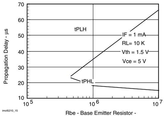
Fig. 15 - Propagation Delay vs. Base Emitter Resistor
