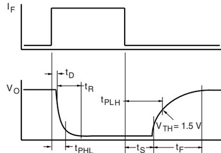
Fig. 2 - Switching Waveform
