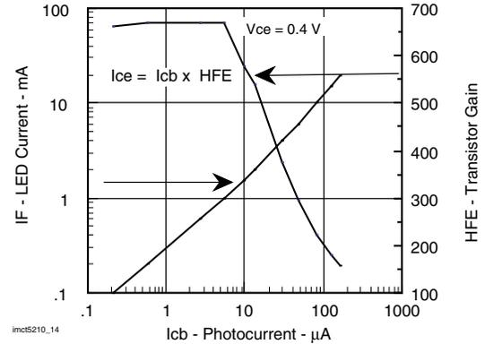
Fig. 14 - Transfer Curve
