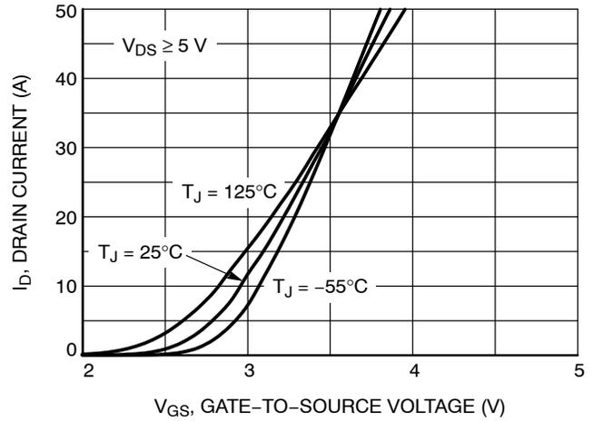
Figure 2. Transfer Characteristics
