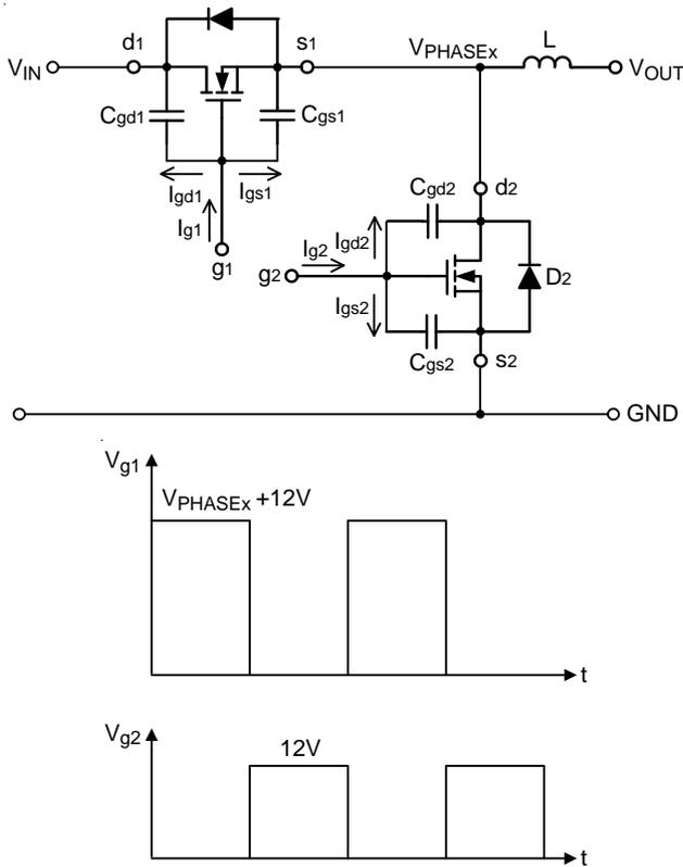
Figure 1. Equivalent Circuit and Waveforms ( $V_{CC} = 12V$ )
