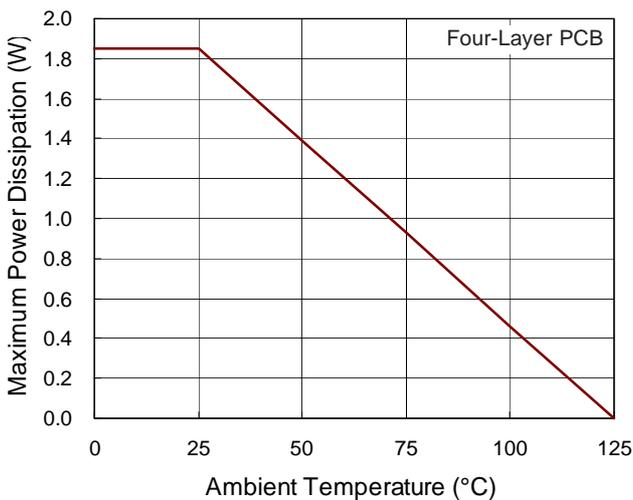
Figure 5. Derating Curve of Maximum Power Dissipation
