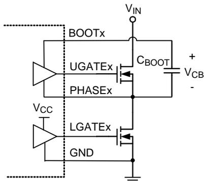
Figure 2. Part of Bootstrap Circuit of RT9625A
