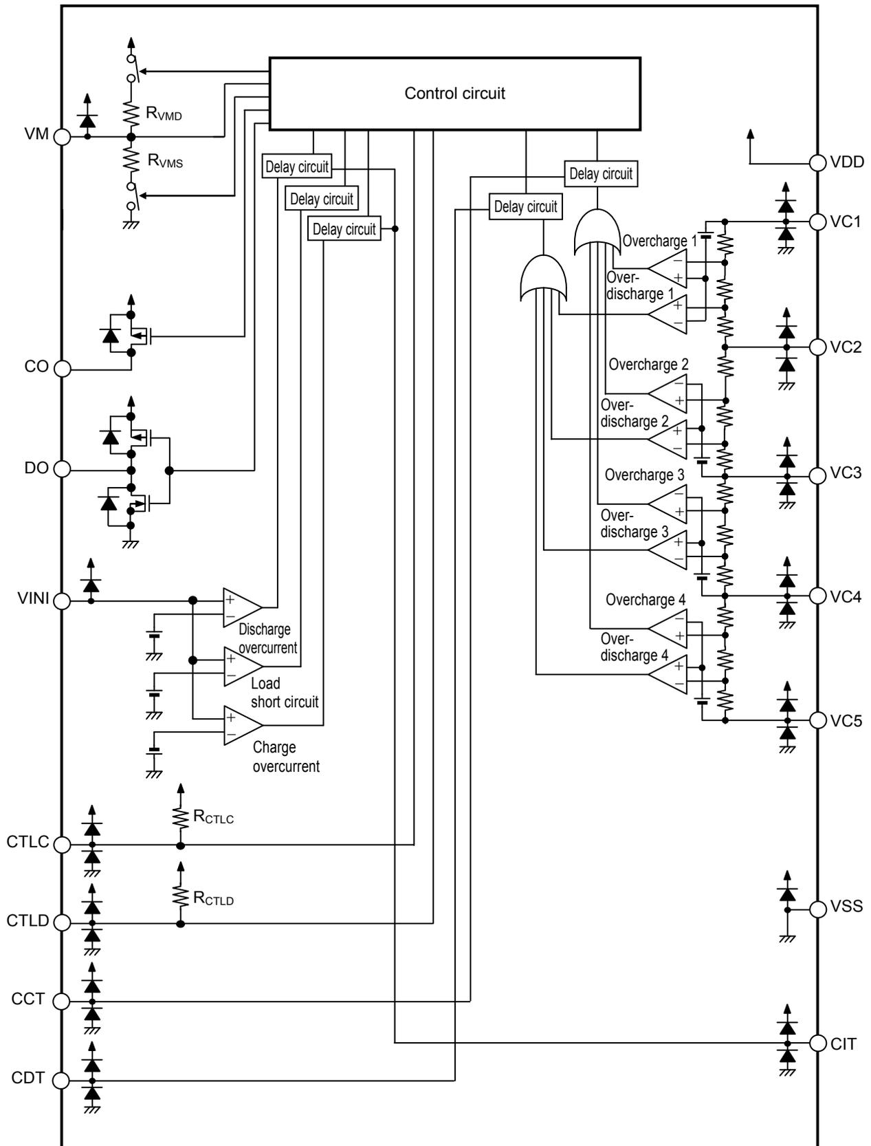
**Remark** Diodes in the figure are parasitic diodes.
