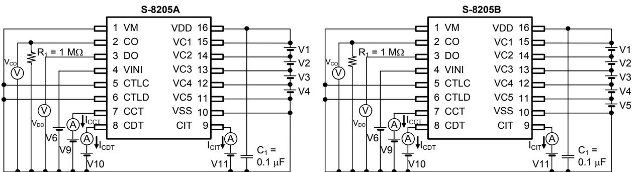
Figure 7 Test Circuit 3
