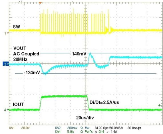
Figure 18: Load Step, DCM / CCM, 0A - 4A - 0A
