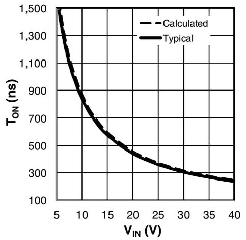
Figure 4:  $T_{ON}$  versus  $V_{IN}$ ,  $R_{ON} = 27.4k\Omega$
