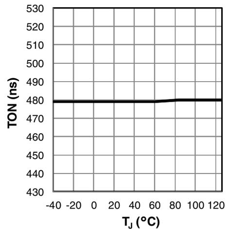
Figure 12:  $T_{ON}$  versus Temperature,  $R_{ON} = 35.7k\Omega$
