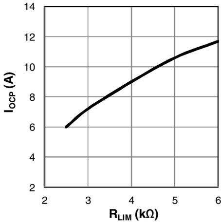
Figure 7: XR76208-Q  $I_{OCP}$  versus  $R_{LIM}$
