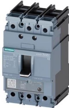
circuit breaker 3VA5 UL frame 125 breaking capacity class M 35kA @ 480 V 3-pole, line protection TM230, FTAM, In=20A overload protection Ir=20A fixed short-circuit protection li=7.5...15 x In UL489 SB (naval), 50 deg. cel. cable connection on both sides
