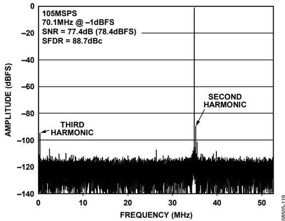
Figure 19. AD9255-105 Single-Tone FFT with  $f_{IN} = 70.1$  MHz
