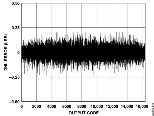
Figure 29. AD9255-105 DNL with  $f_{IN} = 12.5$  MHz
