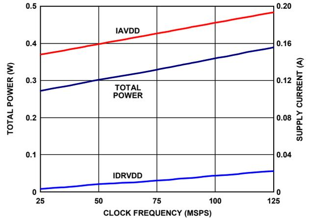
Figure 81. AD9255-125 Power and Current vs. Sample Rate
