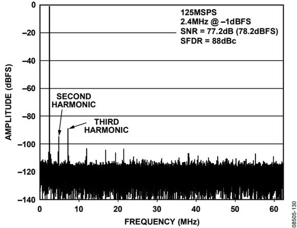
Figure 30. AD9255-125 Single-Tone FFT with  $f_{IN} = 2.4$  MHz
