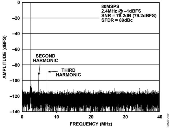
Figure 6. AD9255-80 Single-Tone FFT with  $f_{IN} = 2.4$  MHz
