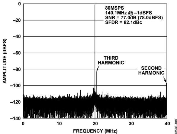
Figure 8. AD9255-80 Single-Tone FFT with  $f_{IN} = 140.1$  MHz
