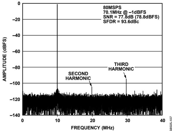
Figure 7. AD9255-80 Single-Tone FFT with  $f_{IN} = 70.1$  MHz
