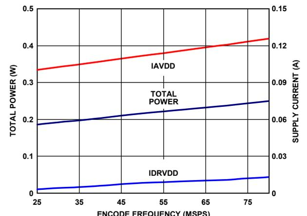
Figure 83. AD9255-80 Power and Current vs. Sample Rate
