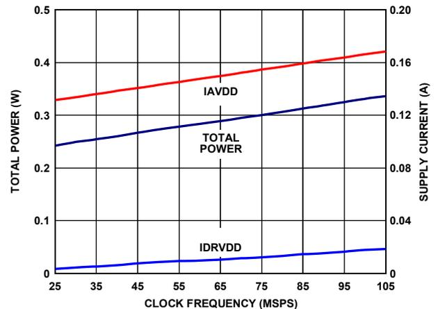
Figure 82. AD9255-105 Power and Current vs. Sample Rate
