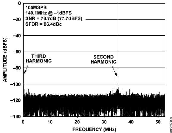
Figure 20. AD9255-105 Single-Tone FFT with  $f_{IN} = 140.1$  MHz
