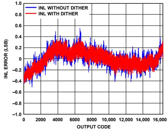
Figure 16. AD9255-80 INL with  $f_{IN} = 12.5$  MHz
