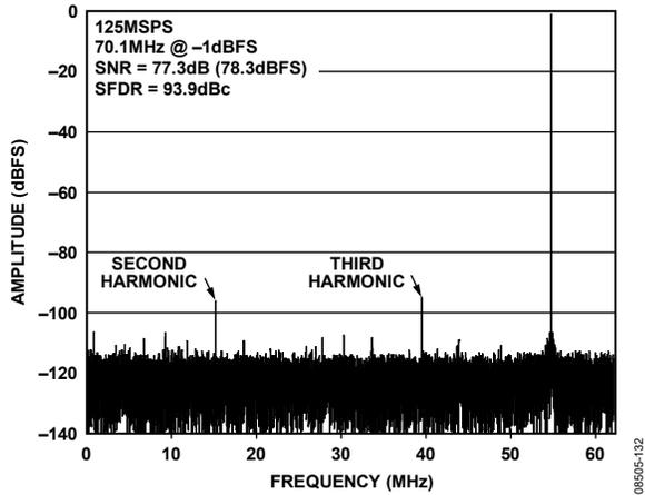
Figure 32. AD9255-125 Single-Tone FFT with  $f_{IN} = 70.1$  MHz
