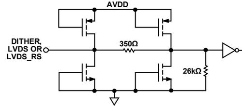
Figure 63. Equivalent DITHER, LVDS, and LVDS\_RS Input Circuit
