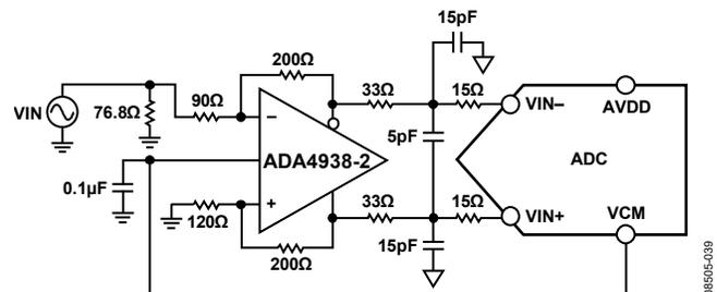
Figure 66. Differential Input Configuration Using the ADA4938-2
