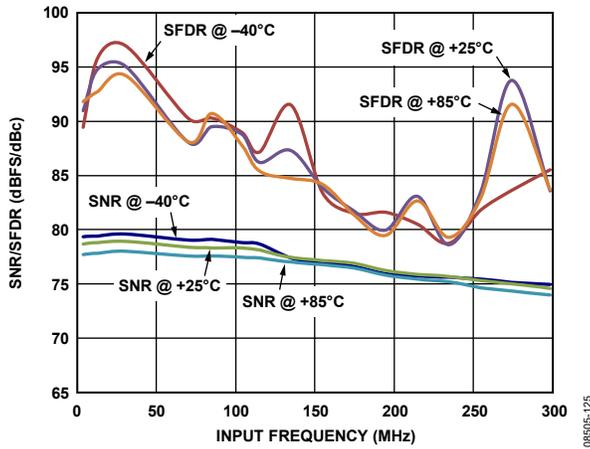
Figure 25. AD9255-105 Single-Tone SNR/SFDR vs. Input Frequency ( $f_{IN}$ ) and Temperature with 2 V<sub>p-p</sub> Full Scale
