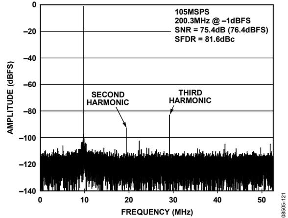
Figure 21. AD9255-105 Single-Tone FFT with  $f_{IN} = 200.3$  MHz
