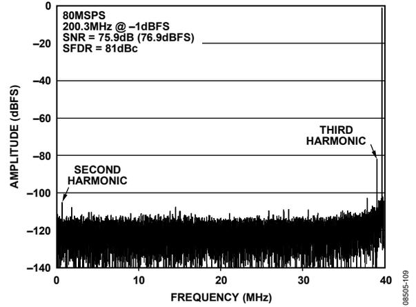
Figure 9. AD9255-80 Single-Tone FFT with  $f_{IN} = 200.3$  MHz
