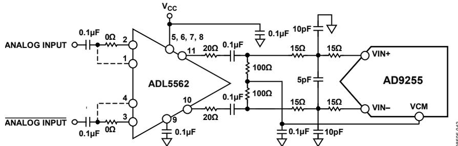
Figure 69. Differential Input Configuration Using the ADL5562
