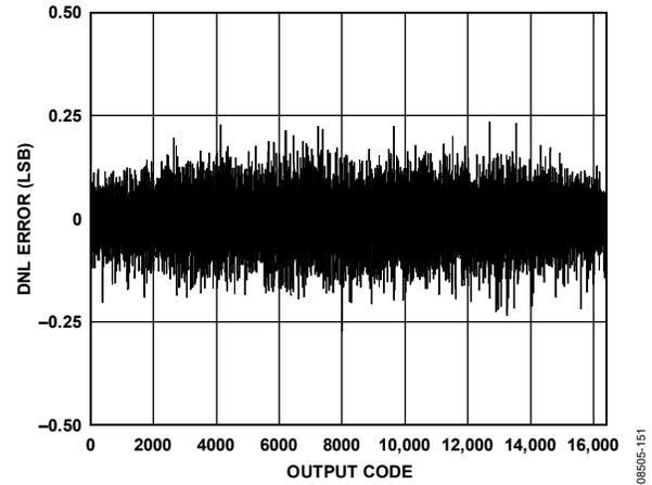
Figure 51. AD9255-125 DNL with  $f_{IN} = 12.5$  MHz
