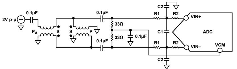
Figure 68. Differential Double Balun Input Configuration
