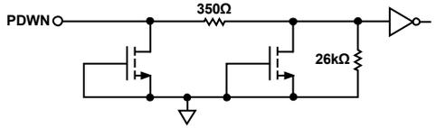
Figure 61. Equivalent PDWN Circuit
