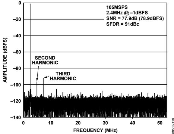
Figure 18. AD9255-105 Single-Tone FFT with  $f_{IN} = 2.4$  MHz
