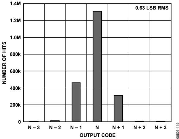
Figure 49. AD9255-125 Grounded Input Histogram
