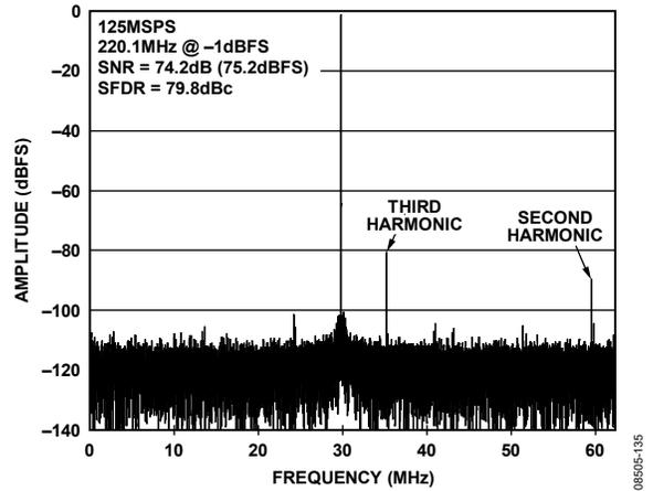
Figure 35. AD9255-125 Single-Tone FFT with  $f_{IN} = 220.1$  MHz
