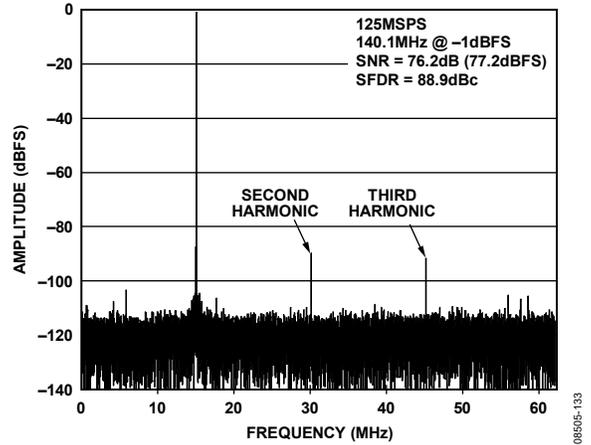
Figure 33. AD9255-125 Single-Tone FFT with  $f_{IN} = 140.1$  MHz
