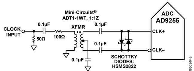
Figure 75. Transformer-Coupled Differential Clock (Up to 200 MHz)
