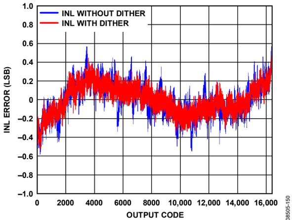
Figure 50. AD9255-125 INL with  $f_{IN} = 12.5$  MHz
