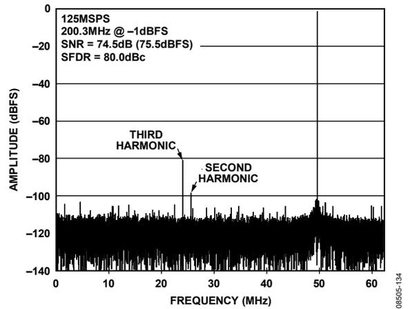
Figure 34. AD9255-125 Single-Tone FFT with  $f_{IN} = 200.3$  MHz
