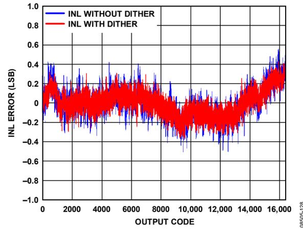
Figure 28. AD9255-105 INL with  $f_{IN} = 12.5$  MHz
