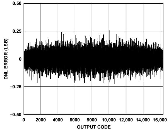
Figure 17. AD9255-80 DNL with  $f_{IN} = 12.5$  MHz
