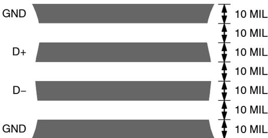
**Figure 19. Arrangement of Signal Tracks**
