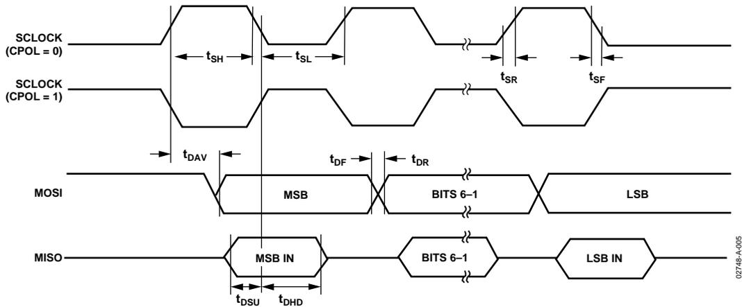
Figure 63. SPI Master Mode Timing (CPHA = 1)
