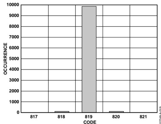
Figure 12. Code Histogram Plot,  $V_{DD} = 3\text{ V}$
