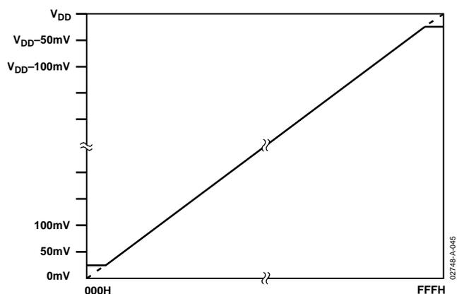
Figure 39. Endpoint Nonlinearities Due to Amplifier Saturation
