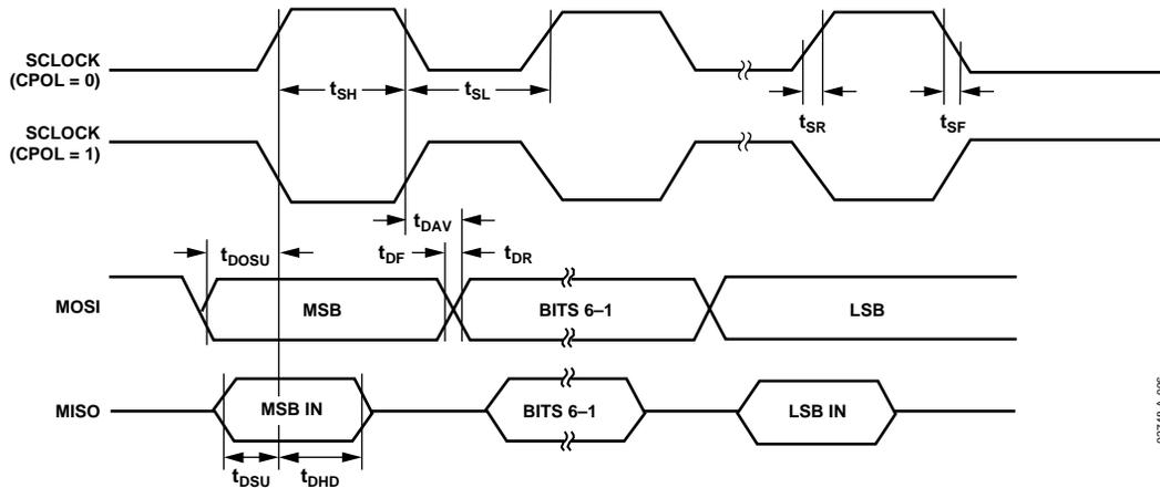
Figure 64. SPI Master Mode Timing (CPHA = 0)
