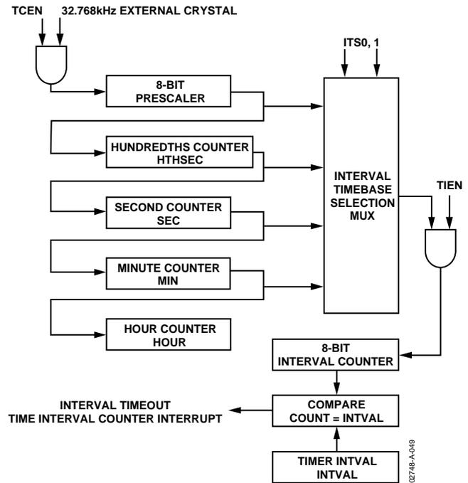
Figure 43. Time Interval Counter, Simplified Block Diagram
