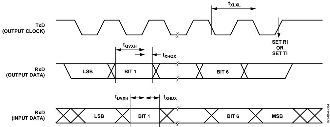
Figure 62. UART Timing in Shift Register Mode
