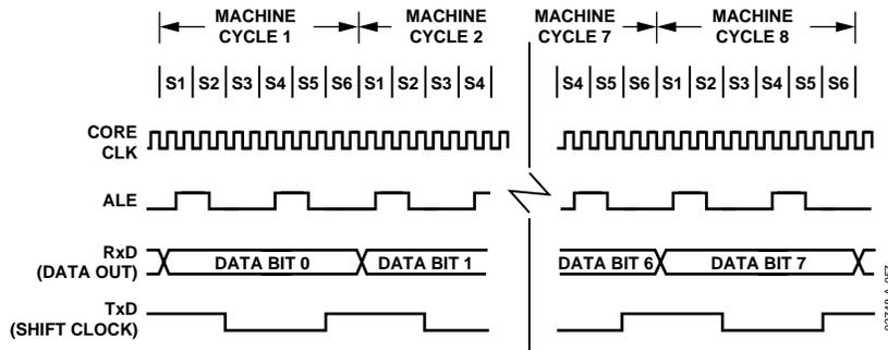
Figure 52. UART Serial Port Transmission, Mode 0
