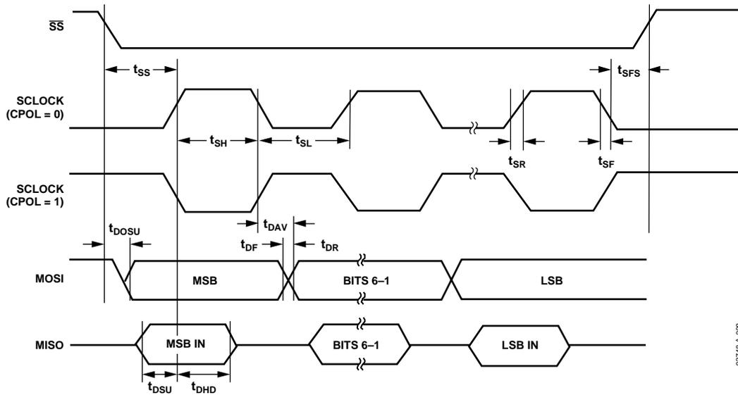
Figure 66. SPI Slave Mode Timing (CPHA = 0)
