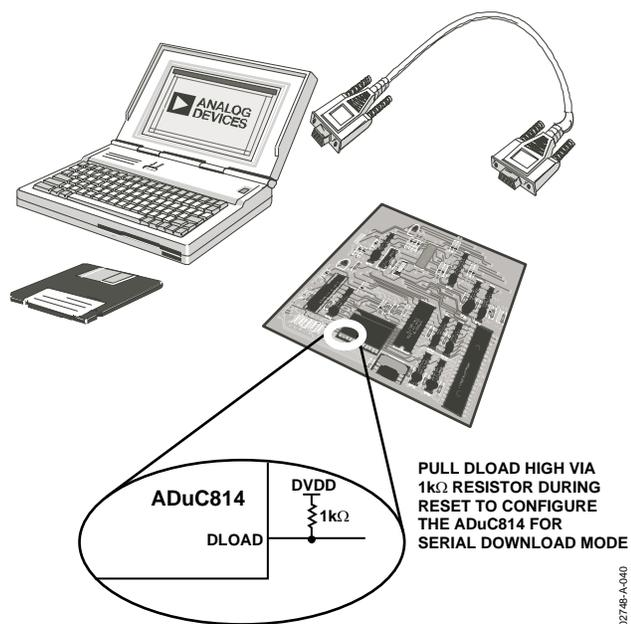
Figure 34. Flash/EE Memory Serial Download Mode Programming
