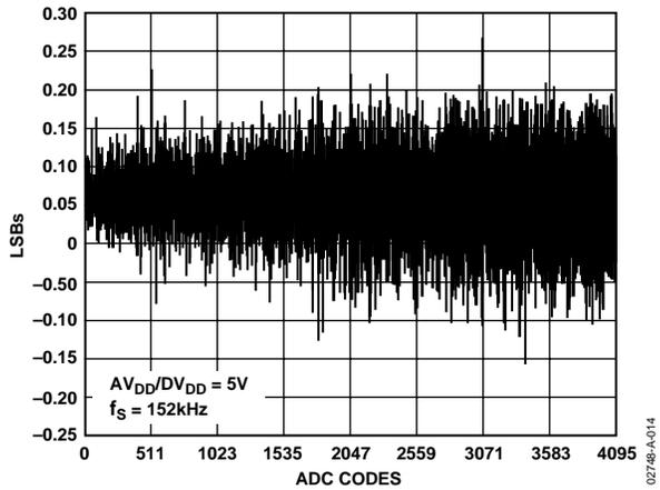
Figure 7. Typical DNL Error,  $V_{DD} = 5\text{ V}$
