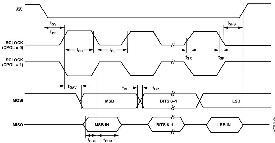
Figure 65. SPI Slave Mode Timing (CPHA = 1)
