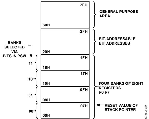
Figure 20. Lower 128 Bytes of Internal Data Memory
