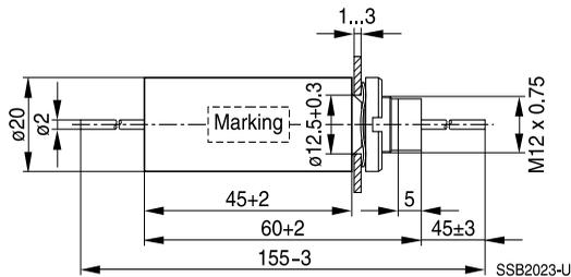
Tightening torque: 4 +0.5 Nm
