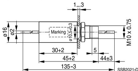
Tightening torque: 3 +0.5 Nm
