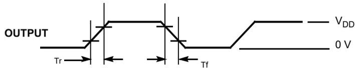
Output Rise time ( $T_r = (0.6 \times V_{DD})/SR1$  (or  $SR3$ )
