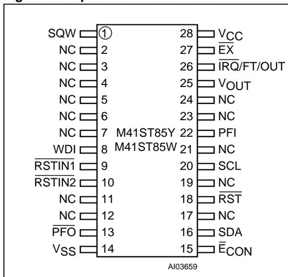
Figure 5. 28-pin, 300mil SOIC (MX) Connections
