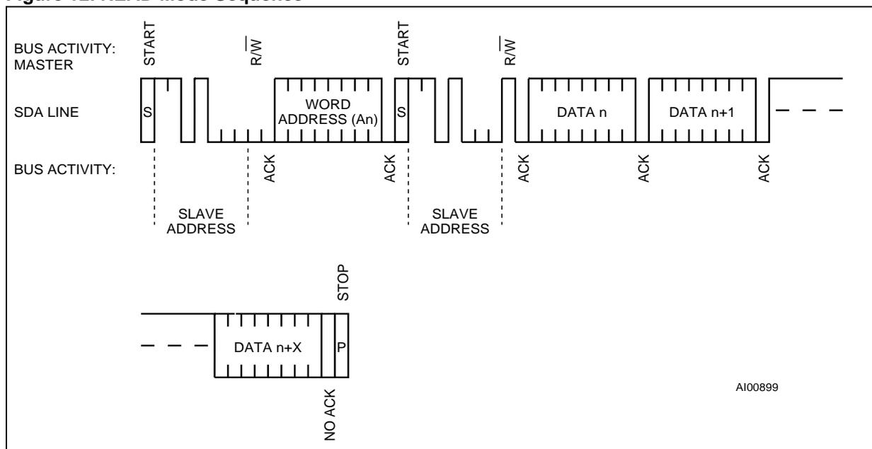
Figure 13. Alternate READ Mode Sequence
