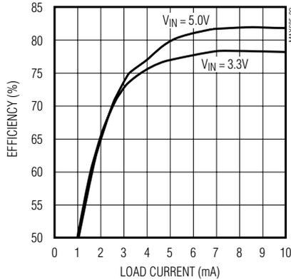
**EFFICIENCY vs. LOAD CURRENT (BOTH OUTPUTS LOADED)**
