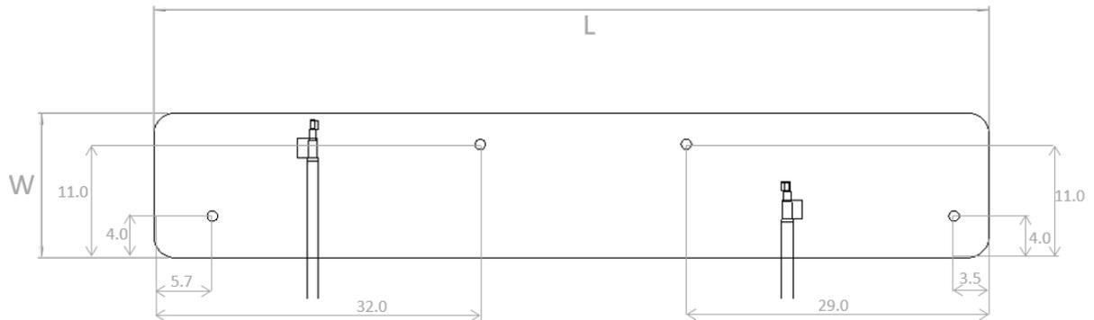
4 Holes = 1mm  $\varnothing$  (diameter)
