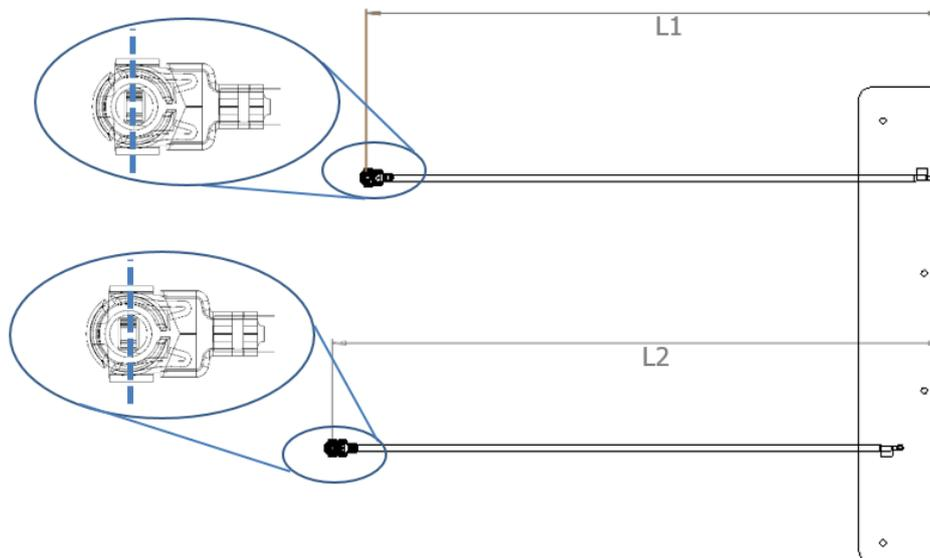
The standard cable length for this antenna is 100mm (other lengths are available, MOQs apply)
