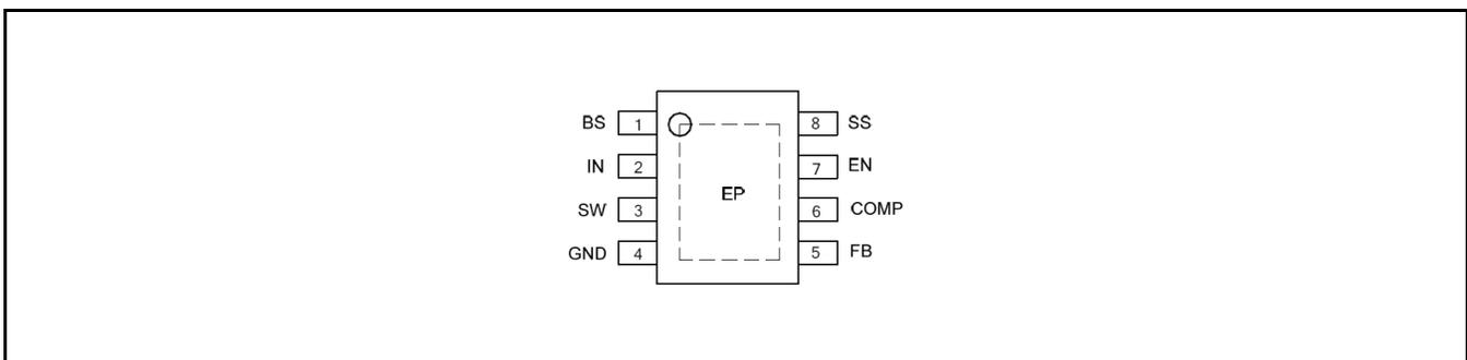
Fig. 3: XRP7665 Pin Assignment (SOIC-8 Exposed Pad)
