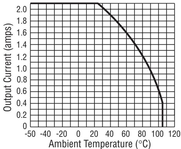
Figure 8 - Maximum Surge Current Without Tripping
