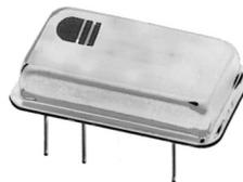
DS11 series SSRs feature state of the art photo-voltaic optical isolation and power MOSFET output chips for ultra-reliable high speed switching of DC loads up to 2 amps, with extremely low on-resistance. Standard options include integral current overload/short circuit protection to provide protection of the relay, load
