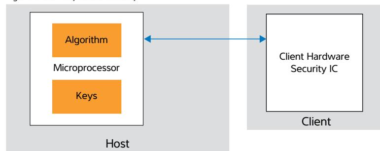
Figure 2. Client and host hardware security
