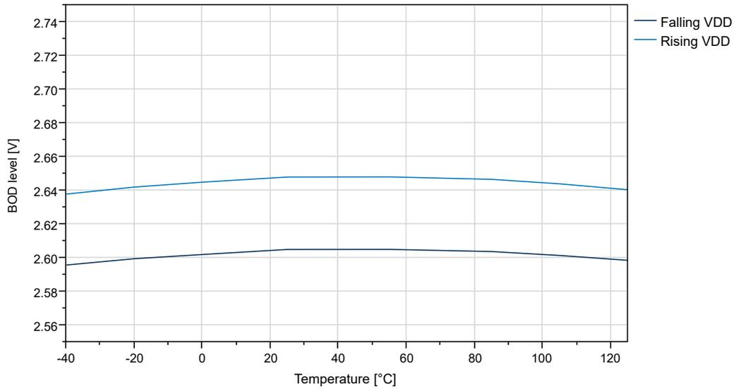
Figure 39-36. BOD Threshold vs. Temperature (Level 4.3V)
