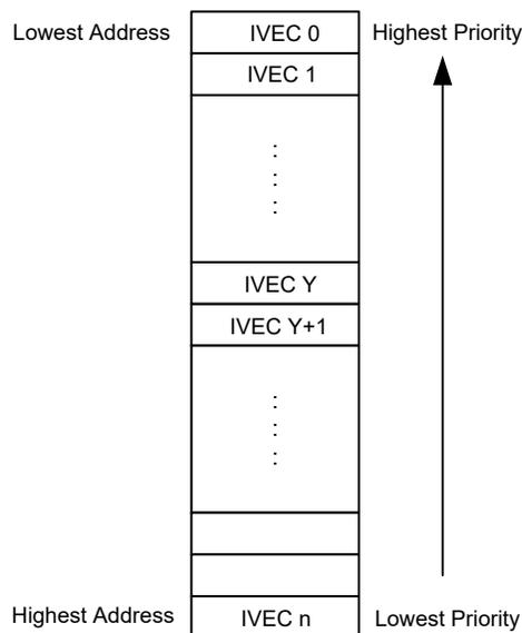
The default priority can be changed by writing to the CPIINT.LVL0PRI register. The value written to the register will identify the vector number with the lowest priority. The next interrupt vector in IVEC will have the highest priority, see the following figure. In this figure, the value Y has been written to
