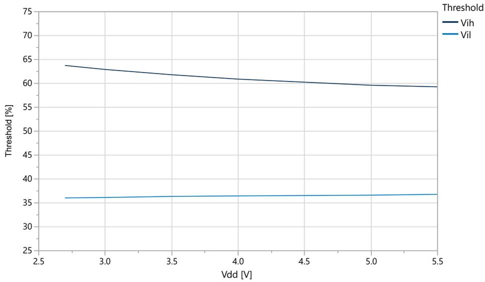
Figure 39-18. I/O Pin Input Threshold Voltage vs.  $V_{DD}$  ( $V_{IH}$ )
