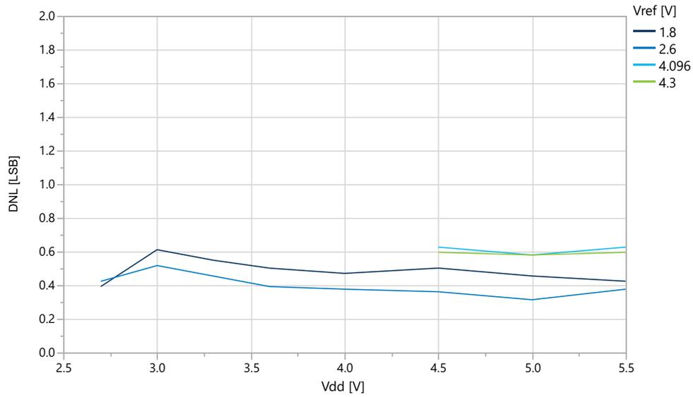
**Figure 39-50. DNL vs.  $V_{REF}$  ( $V_{DD}=5.0\text{V}$ ,  $f_{ADC}=115$  ksp/s, REFSEL = External Reference)**
