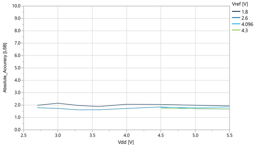
**Figure 39-48. Absolute Accuracy vs.  $V_{REF}$  ( $V_{DD}=5.0\text{V}$ ,  $f_{ADC}=115$  ksp/s, REFSEL = External Reference)**
