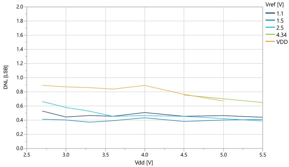
**Figure 39-40. DNL vs.  $V_{ref}$  ( $V_{DD}=5.0\text{V}$ ,  $f_{ADC}=115$  ksp/s), REFSEL = Internal Reference**
