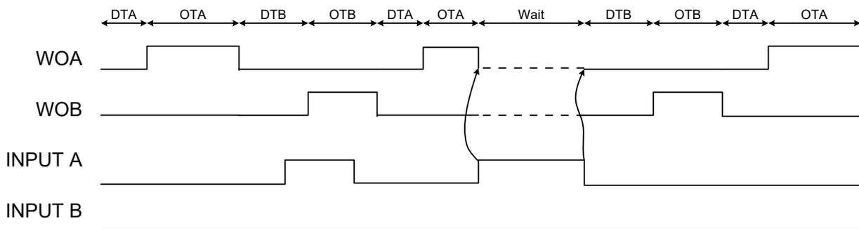
If Input mode 1 is used on input B, an event will only have an effect if the TCD is in Dead-time B or On-time B, and it will only affect the output WOB. When the event is done, the TCD counter starts at Dead-time A.
