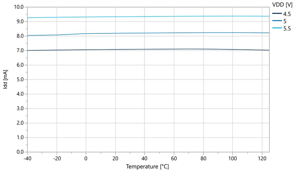
Figure 39-4. Active Supply Current vs.  $V_{DD}$  (f=[1, 16] MHz OSC20M) at T=25°C
