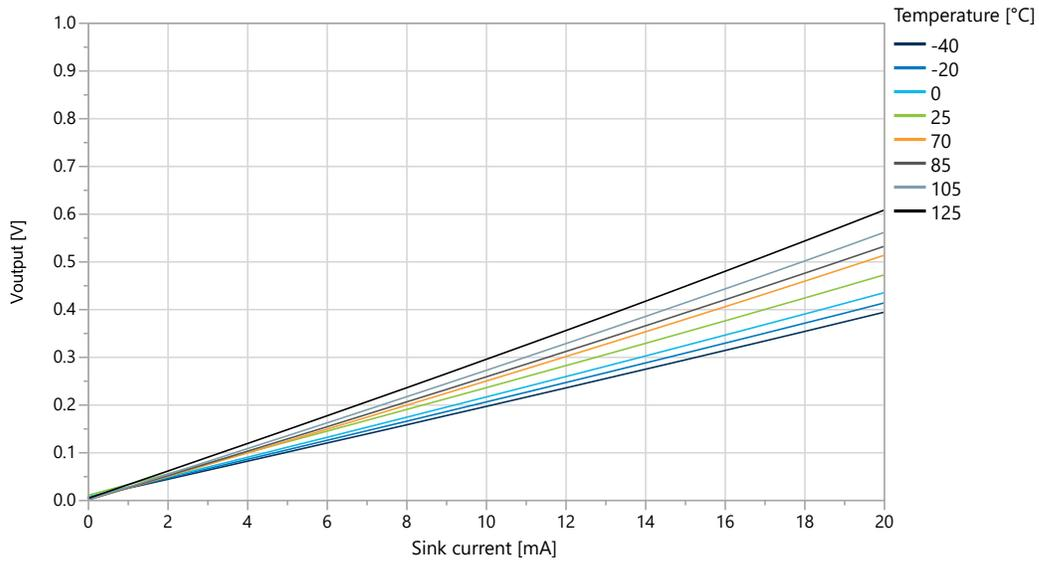
Figure 39-22. I/O Pin Output Voltage vs. Sink Current ( $T=25^{\circ}C$ )
