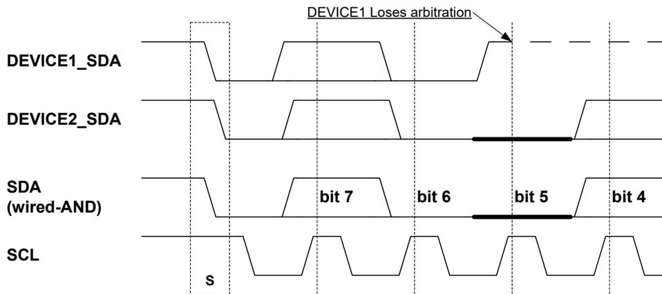
Figure 27-10 shows an example where two TWI masters are contending for bus ownership. Both devices are able to issue a Start condition, but DEVICE1 loses arbitration when attempting to transmit a high level (bit 5) while DEVICE2 is transmitting a low level.
