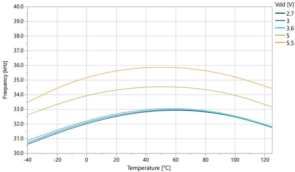
**Figure 39-70. OSCULP32K Internal Oscillator Frequency vs. V<sub>DD</sub>**
