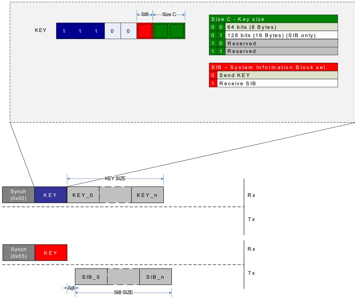
The figure above shows the transmission of a KEY and the reception of a SIB. In both cases, the `SIZE_C` field in the opcode determines the number of frames being sent or received. There is no response after sending a `KEY` to the UPDI. When requesting the SIB, data will be transmitted from the UPDI according to the current Guard Time setting.
