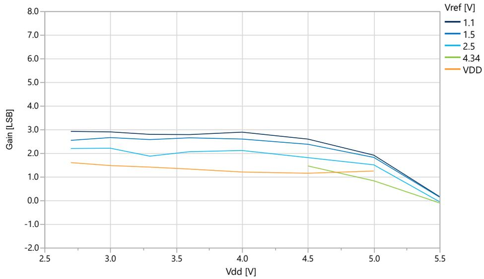
**Figure 39-42. Gain Error vs.  $V_{ref}$  ( $V_{DD}=5.0\text{V}$ ,  $f_{ADC}=115$  kpsps), REFSEL = Internal Reference**
