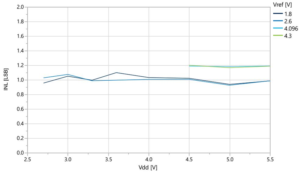
**Figure 39-54. INL vs.  $V_{REF}$  ( $V_{DD}=5.0\text{V}$ ,  $f_{ADC}=115$  ksp/s, REFSEL = External Reference)**
