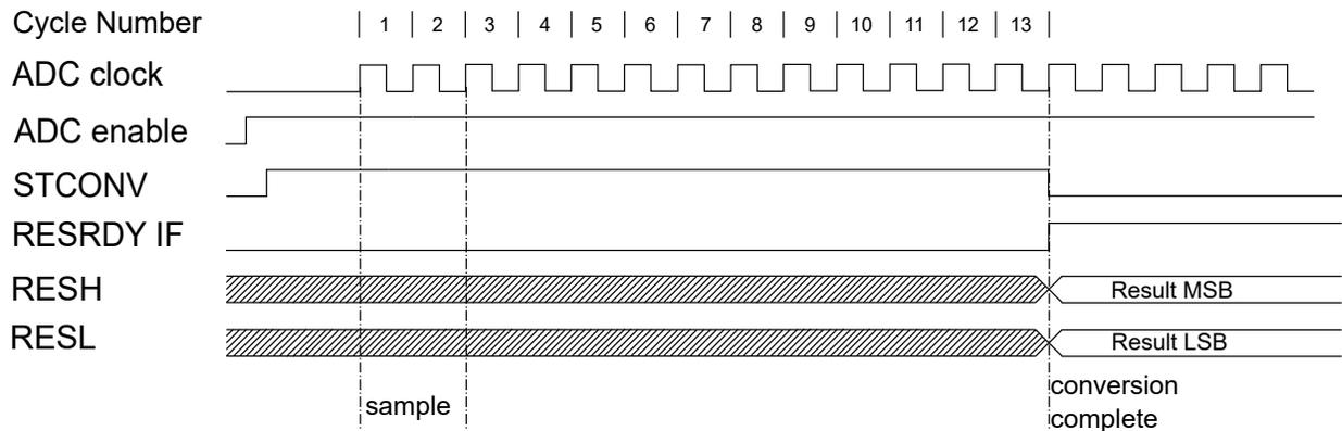
Both sampling time and sampling length can be adjusted using the Sample Delay bit field in Control D (ADC.CTRLD) and sampling the Sample Length bit field in the Sample Control register (ADC.SAMPCTRL). Both of these control the ADC sampling time in a number of CLK\_ADC cycles. This allows sampling high-impedance sources without relaxing conversion speed. See the register description for further information. Total sampling time is given by:
