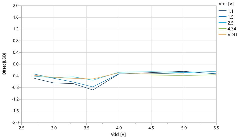
**Figure 39-46. Offset Error vs.  $V_{ref}$  ( $V_{DD}=5.0\text{V}$ ,  $f_{ADC}=115$  kps), REFSEL = Internal Reference**
