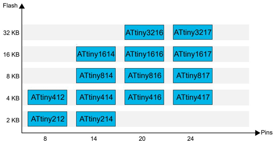
Devices with different Flash memory size typically also have different SRAM and EEPROM.
