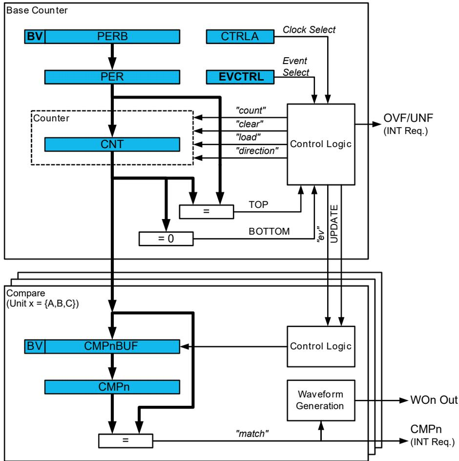
The counter register (TCA<sub>n</sub>.CNT), period registers with buffer (TCA<sub>n</sub>.PER and TCA<sub>n</sub>.PERBUF), and compare registers with buffers (TCA<sub>n</sub>.CMP<sub>x</sub> and TCA<sub>n</sub>.CMPBUF<sub>x</sub>) are 16-bit registers. All buffer registers have a buffer valid (BV) flag that indicates when the buffer contains a new value.
