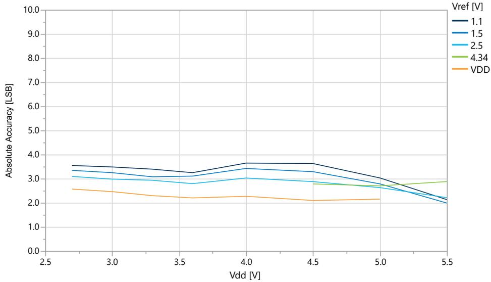
**Figure 39-38. Absolute Accuracy vs.  $V_{ref}$  ( $V_{DD}=5.0\text{V}$ ,  $f_{ADC}=115$  ksp/s), REFSEL = Internal Reference**
