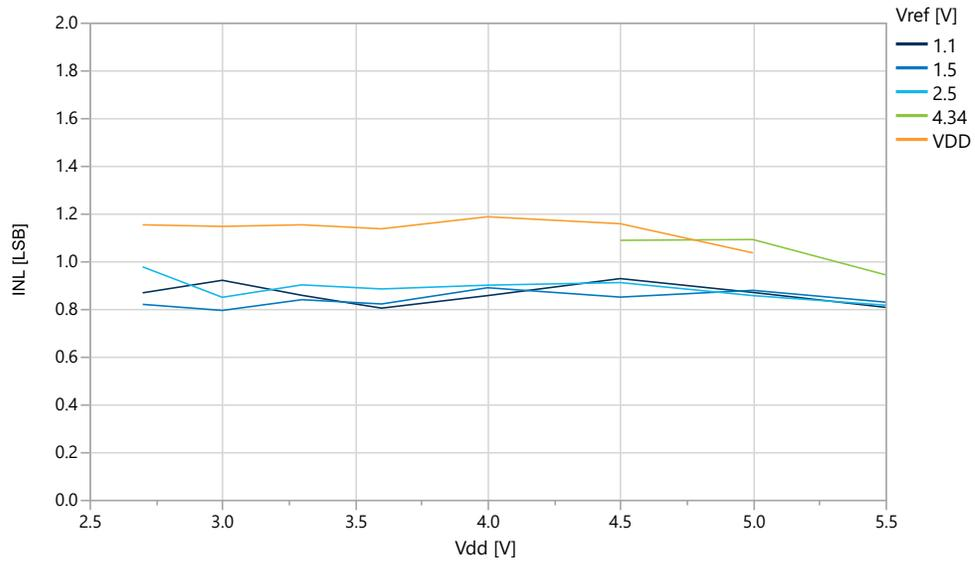
**Figure 39-44. INL vs.  $V_{ref}$  ( $V_{DD}=5.0\text{V}$ ,  $f_{ADC}=115$  kps), REFSEL = Internal Reference**
