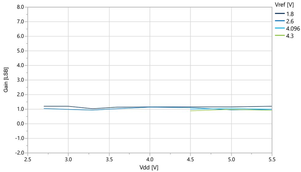
**Figure 39-52. Gain vs.  $V_{REF}$  ( $V_{DD}=5.0\text{V}$ ,  $f_{ADC}=115$  ksp/s, REFSEL = External Reference)**
