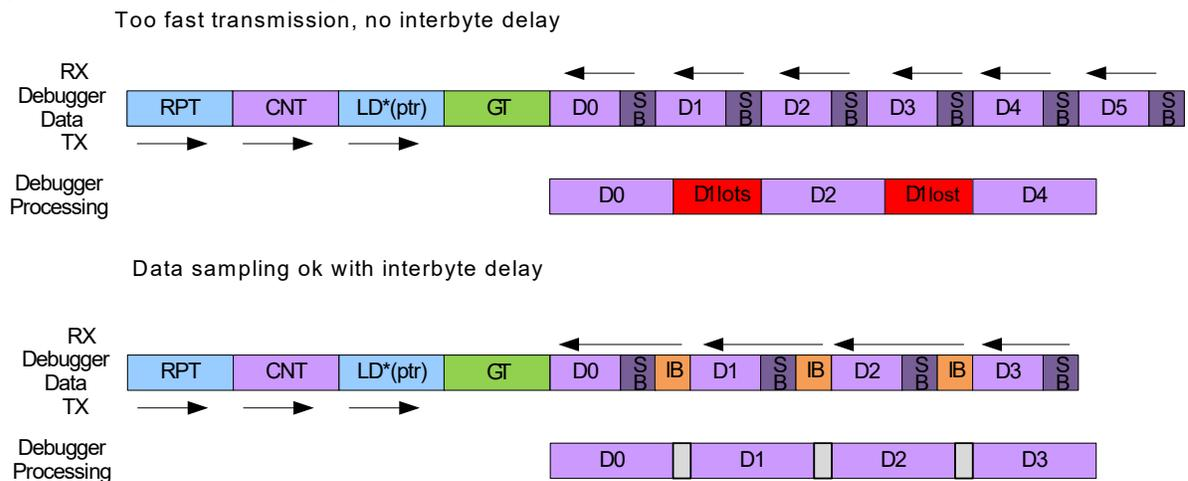
In Figure 34-18, GT denotes the Guard Time insertion, SB is for Stop Bit and IB is the inserted interbyte delay. The rest of the frames are data and instructions.
