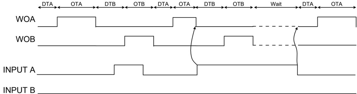
If Input mode 2 is used on input B, an event will only have an effect if the TCD is in Dead-time B or On-time B, and it will only affect the output WOB.
