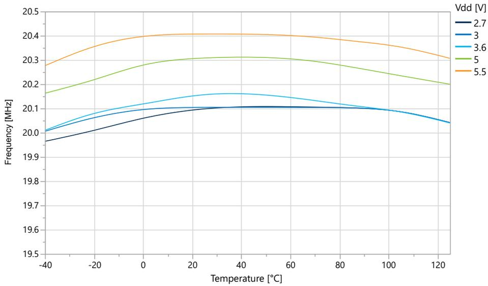
Figure 39-68. OSC20M Internal Oscillator: Frequency vs. V<sub>DD</sub>
