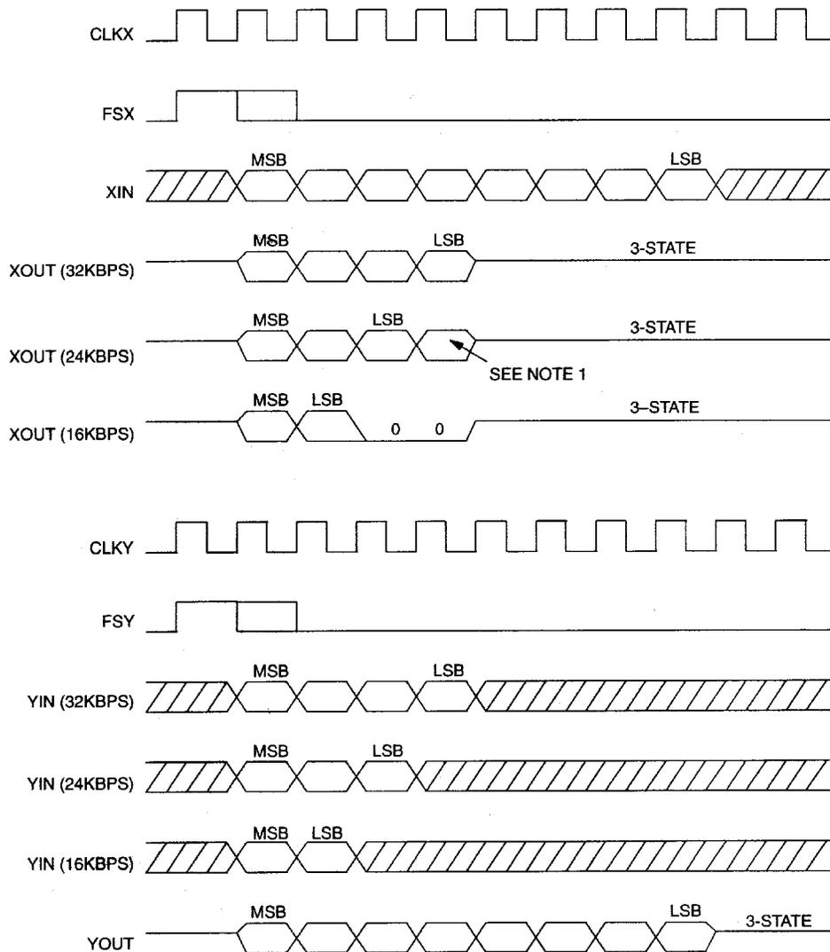
**Note 1:** The bit after the LSB in the 24kbps ADPCM output is only a 1 when the DS2164Q is operated in the software mode and is programmed to perform 24kbps compression; in all other configurations, it is a 0.
