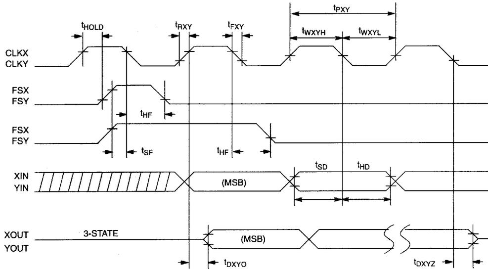
**Figure 14. MASTER CLOCK/RESET AC TIMING DIAGRAM**
