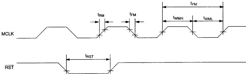
**Figure 15. SERIAL PORT AC TIMING DIAGRAM**
