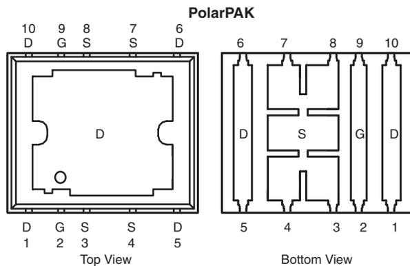
Top surface is connected to pins 1, 5, 6, and 10
