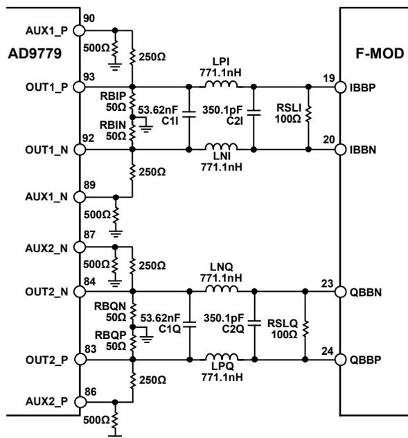
Figure 34. DAC Modulator Interface with Auxiliary DAC Resistors
