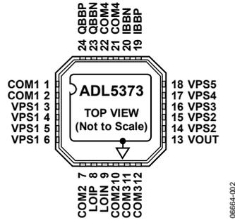
Figure 2. Pin Configuration
