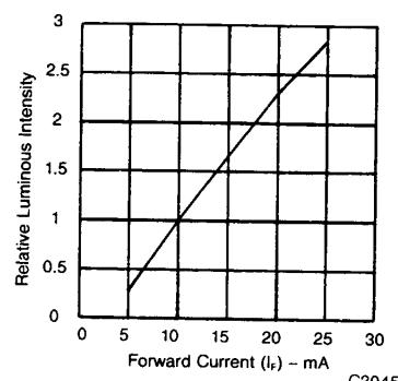
Fig. 3. Relative Luminous Intensity vs.
