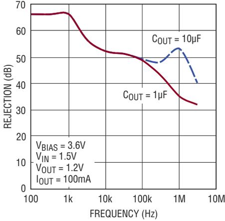
**BIAS Ripple Rejection vs Frequency**
