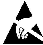
**ESD (electrostatic discharge) sensitive device.**
