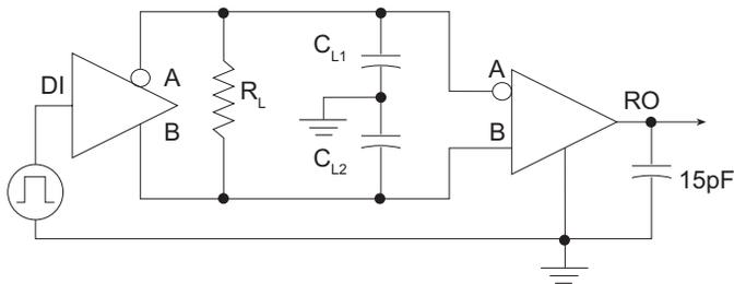
Figure 3. Driver / Receiver Timing Test Circuit
