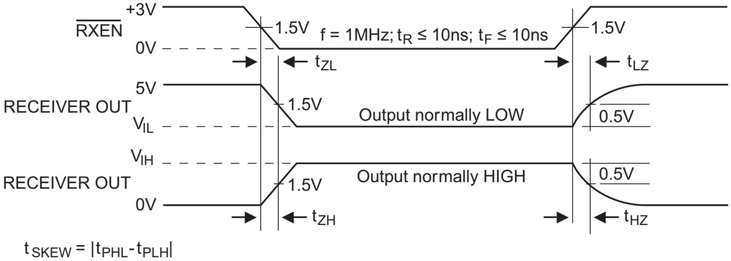
$$t_{\text{SKEW}} = |t_{\text{PHL}} - t_{\text{PLH}}|$$
