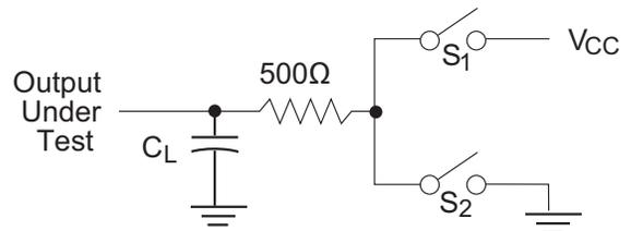
Figure 4. Driver Timing Test Load #2 Circuit
