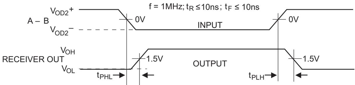
Figure 7. Receiver Propagation Delays
