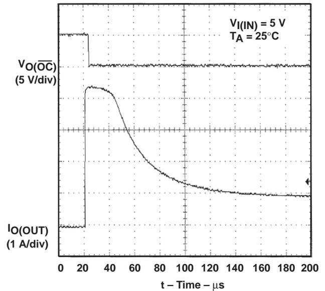
Figure 11. 1- $\Omega$  Load Connected to Enabled Device
