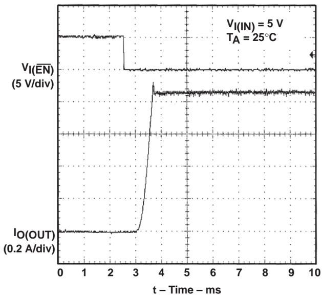
Figure 6. TPS2042, Short-Circuit Current, Device Enabled into Short
