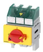
SENTRON, Molded case switch 3LD5 UL, Emergency switching-off, 3-pole, certified according to UL489 UL60947-4-1 and IEC60947-3, UL: 30A, SCCR 50kA at 480VAC, Operating power at 480VAC 3-phase: 20hp, IEC: 32A, Operating power at AC-23A at 400V: 15kW, floor mounting with direct handle, red/yellow, incl. terminal covers for the infeed side
