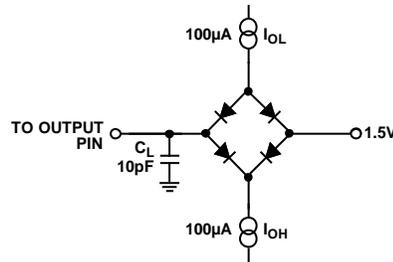
Figure 4. Load Circuit for MUXOUT Timing, C<sub>L</sub> = 10 pF
