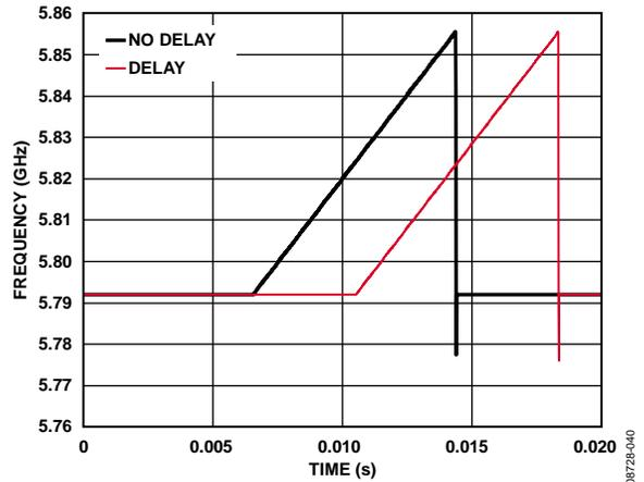
Figure 10. Delayed Start of Triangular Burst, PFD = 32 MHz, INT = 181, FRAC = 0, DEV Offset = 4, DEV Word = 20972, Step Word = 200, CLK<sub>2</sub> Divider = 10, CLK<sub>1</sub> Divider = 125, DEL Start Word = 1000
