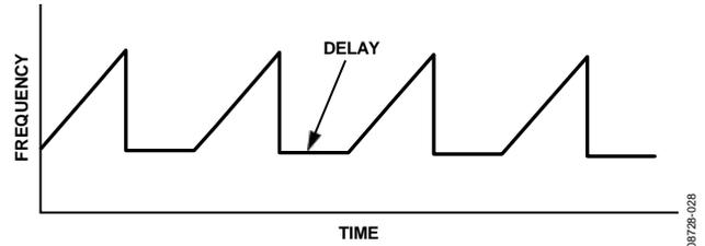
Figure 39. Delay Between Ramps for Sawtooth Mode
