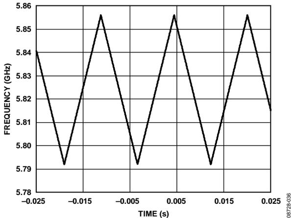
Figure 7. Triangular Waveform, PFD = 32 MHz, INT = 181, FRAC = 0, DEV Offset = 4, DEV Word = 20972, Step Word = 200, CLK<sub>2</sub> Divider = 10, CLK<sub>1</sub> Divider = 125
