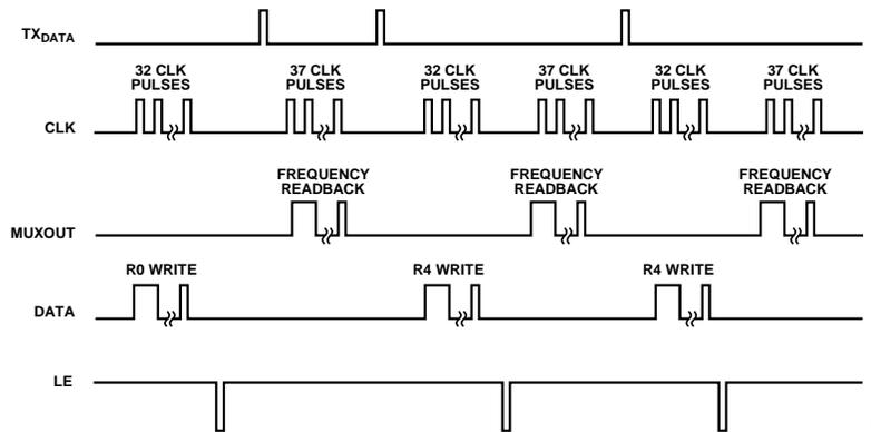
Figure 45. Continuous Frequency Readback
