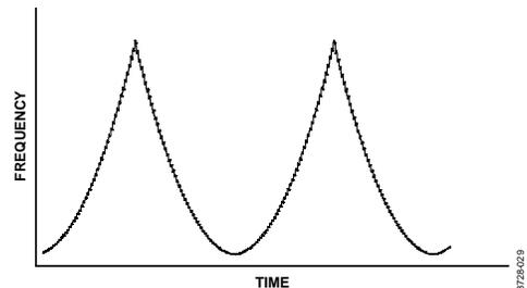
Figure 40. Parabolic Ramp
