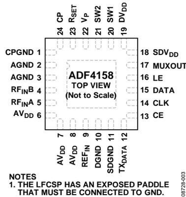
Figure 5. Pin Configuration
