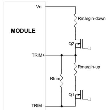
Figure 26. Circuit Configuration for margining Output voltage.
