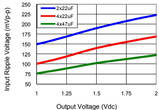
Figure 22. Input ripple voltage for various output voltages with  $2 \times 22\mu\text{F}$ ,  $4 \times 22\mu\text{F}$  or  $4 \times 47\mu\text{F}$  ceramic capacitors at the input (maximum load). Input voltage is 12V
