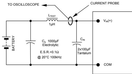
NOTE: Measure input reflected ripple current with a simulated source inductance ( $L_{TEST}$ ) of  $1\mu\text{H}$ . Capacitor  $C_S$  offsets possible battery impedance. Measure current as shown above.
