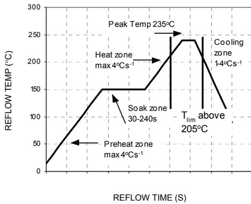
Figure 32. Reflow Profile for Tin/Lead (Sn/Pb) process.
