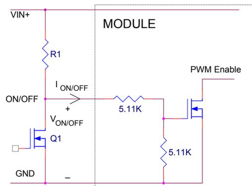
**Figure 24. Remote On/Off Implementation using ON/OFF .**
