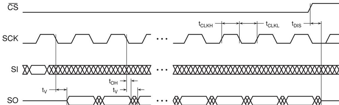
Figure 16-3.  $\overline{WP}$  Timing for Write Status Register Byte 1 Command When SPRL = 1
