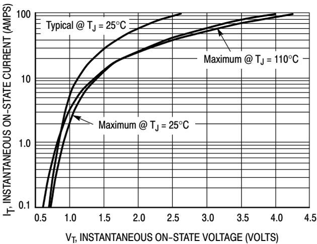
Figure 3. On-State Characteristics
