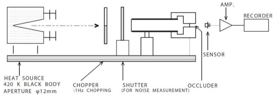
**Figure 2 - Occluder Position**
